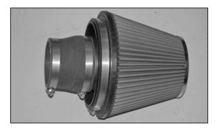
18. Install the silicone hose (08724) onto the filtercharger assembly and secure with the provided hose clamp as shown.
