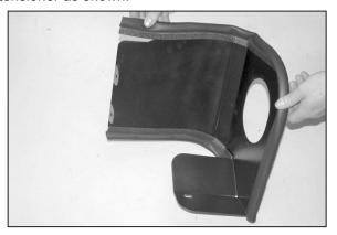
9. Install the edge trim seal onto the heat shield as shown.
