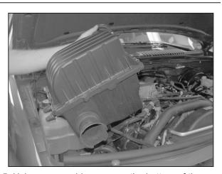
5. Using a screwdriver, pry up the bottom of the air cleaner to release the air cleaner from the mounting grommets, and then remove the air cleaner assembly as shown.
