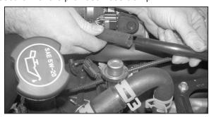
16. Cut the factory crank case vent tube one inch from the end, then attach the supplied silicone vent hose to the K&N® intake tube and factory vent tube as shown.
