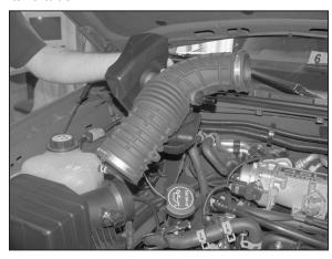
4. Loosen the hose clamps at the throttle body and the air box, and then remove the stock intake tube as shown.
