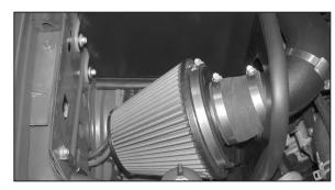
19. Install the filtercharger assembly onto the K&N® intake tube and secure with the provided hose clamp as shown.
