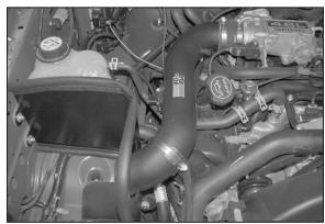
15. Install the K&N® intake into the silicone hose at the throttle body and onto the saddle clamp, then secure with the provided hose clamp.
