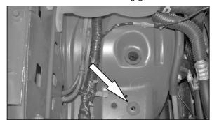
11. Install the inserted nut into the forward air box mounting grommet hole vacated in step #10 as shown.
