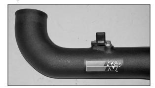
14. Install the mass <u>air sensor</u> into the K&N® intake tube and secure with the factory screws and spacers provided.
