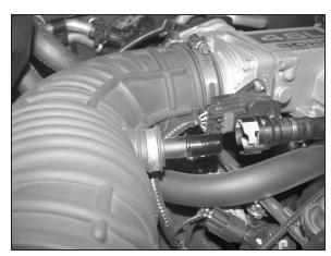
3. Release the green locking tab and then disconnect the crank case vent from the stock intake tube.
