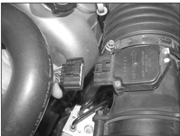
2. Disconnect the mass air sensor electrical connection.
