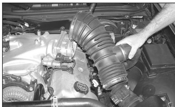
4. Loosen the two hose clamps which secure the stock intake tube to the throttle body and mass air sensor and then remove the intake tube from the vehicle as shown.
