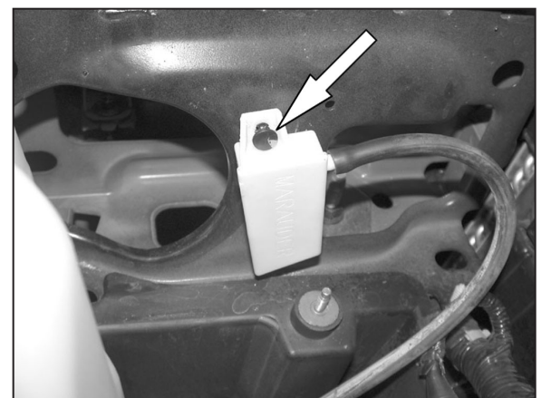
7. Remove the air compressor muffler-retaining pin shown and then remove the muffler from the core support.
