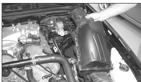
6. Lift and remove the air box from the vehicle as shown. NOTE: K&N Engineering, Inc., recommends that customers do not discard factory air intake.
