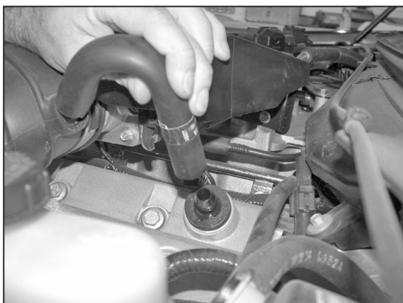
3. Disconnect the crank case vent hose from the valve cover vent fitting as shown.
