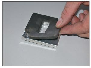
20. Install the provided gasket onto the K&N $^{\mbox{\tiny \$}}$  mass air adapter as shown.
