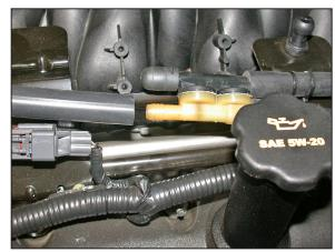
27. Install the supplied 3/8" vent hose onto the K&N<sup>®</sup> intake tube, and then connect the open end to the evaporative valve as shown.
