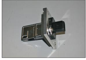
21. Using the screws removed in step #19, install the mass air sensor into the K&N $^{\odot}$  mass air adapter.
