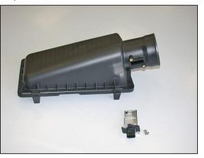
19. Using the "TORX" wrench provided, remove the mass air sensor from the air box lid as shown.
