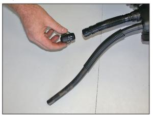
24. Pull firmly on the crank case vent elbow to remove from the vent tube as shown.
