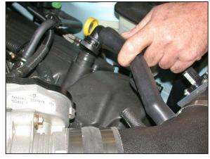
26. Install the vent hose assembly onto the K&N<sup>®</sup> intake tube and then snap the vent elbow onto the valve cover as shown.
