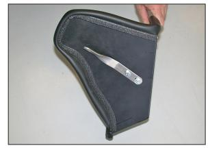
12. Install the heat shield mounting bracket (010083) onto the heat shield as shown with the provided hardware.
