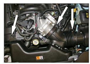
7. Loosen the hose clamps at the throttle body and the factory air box, and then remove the intake tube retaining nut shown.
