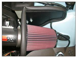
29. Install the K&N<sup>®</sup> air filter and secure with the provided hose clamp.
