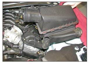
10. Pull up firmly on the air box to dislodge it from the retaining pin, and then remove the air box from the vehicle.
