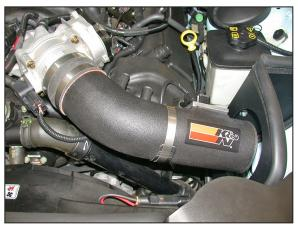
23. Install the K&N<sup>®</sup> intake tube assembly into the silicone hose at the throttle body and onto the
