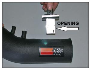
22. Install the mass air assembly into the K&N $^{\odot}$  intake tube and secure with the provided hardware.
