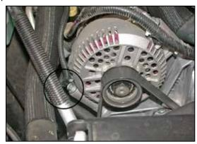
17. Remove the front lower alternator mounting bolt shown.
