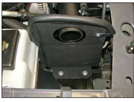
22. Install the heat shield assembly into the vehicle so the bracket lines up with the factory in the core support and the heat shield holes line up with the threaded inserts installed in step #21.
