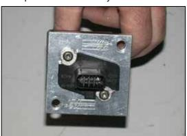
13. Using the factory mounting screws, install mass air sensor into the  $K\&N^{\otimes}$  adapter assembly as shown.
