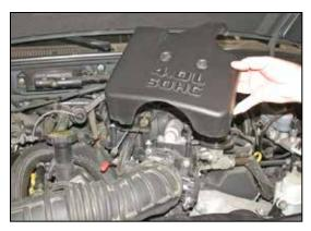
4. Remove the engine cover from the engine.
