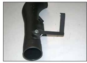
16. Install the provided tube-mounting bracket (010081) onto the K&N® intake tube with the provided hardware as shown.
