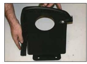
20. Install the provided edge trim onto the heat shield as shown.
