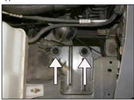
9. Remove the two-airbox mounting grommets from the mounting plate shown.
