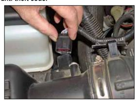
2. Depress the locking tab on the mass air sensor electrical connection and then disconnect the electrical connection and separate the harness from the stock intake tube wiring harness clip.
