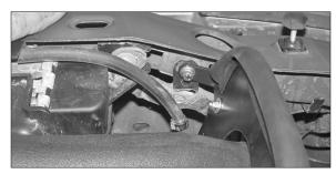
23. Fasten the heat shield mounting bracket to the core support with the bolt and lock washer provided passing through the wiring harness mount into the core support as shown.
