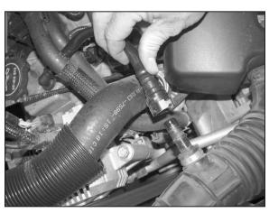
3. Rotate the green locking tab counter clockwise and then disconnect the crankcase vent from the intake tube as shown.
