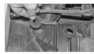
14. Remove the two airbox mounting grommets from the airbox mounting bracket as shown.
