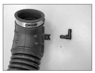
3b. Cut the clamp which secures the 90° fitting to the stock intake hose and then remove the fitting as shown.
