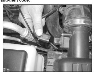
2. Disconnect the mass air electrical connection, and then disconnect wiring harness from intake tube.
