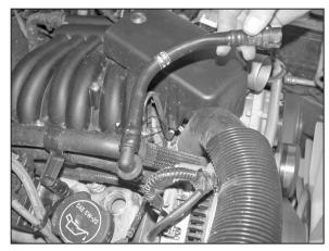
5. Remove crankcase vent tube from valve cover as shown.
