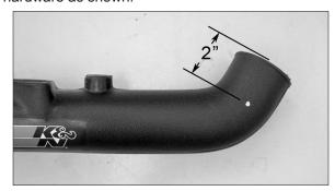
10a. On vehicles equipped with a brake booster breather line, measure 2.0" from the outlet end of the tube and mark the location to be drilled.
