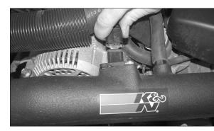
29. Reconnect the mass air electrical connection as shown.
