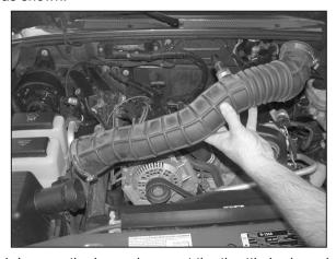
4. Loosen the hose clamps at the throttle body and the factory airbox, and then remove the intake tube from the vehicle as shown.
