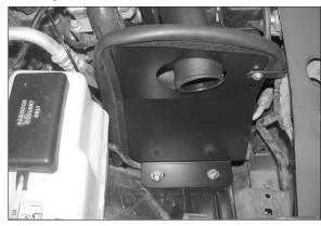
22. Install the heat shield into the vehicle using the 3/8" bolts and washers provided threaded into the inserts installed in step #21.
