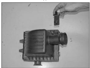
8. Remove the two mass air retaining screws with the torx wrench provided, and then remove the mass air sensor as shown.
