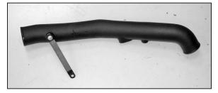
10. Mount the tube-mounting bracket (010078) onto the new K&N<sup>®</sup> intake tube with the provided hardware as shown.
