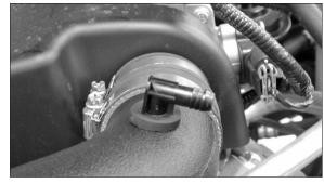
16a. On vehicles equipped with a brake booster bretaher line, install the factory 90° fitting removed in step #3b into the grommet installed into the K&N® intake tube in step #10b.
