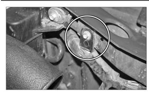
18. Remove the wiring harness mounting bolt shown from the radiator core support.
