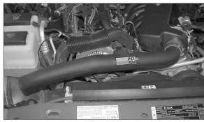
16. Install the intake tube onto the throttle body, then using the bolt removed in step #9 secure the bracket onto the alternator as shown.
