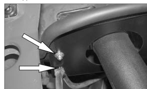
24. Attach the coolant reservoir house clip to the heat shield as shown.
