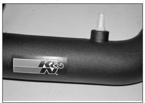
11. Install the vent fitting into the new intake tube as shown.
