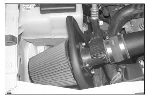
19. Install the K&N® filtercharger onto the mass air assembly as shown.
