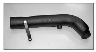
10. Mount the provided bracket onto the new K&N<sup>®</sup> intake tube with the provided hardware as shown.
