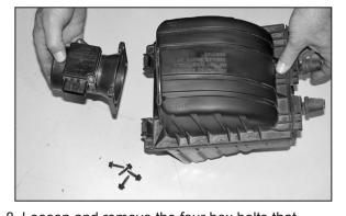
8. Loosen and remove the four hex bolts that secure the mass air sensor, then, remove the mass air sensor from the air cleaner as shown.
