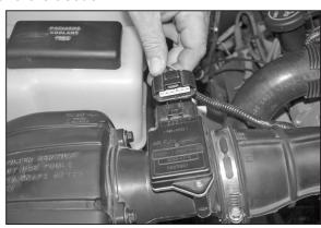
2. Disconnect the mass air electrical connection, then disconnect wiring harness from intake tube.
