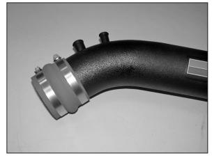
19. Install the provided silicone hump hose (087121) onto the K&N $^{\circ}$  intake tube with the provided hose clamps.
