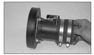
24. Install the silicone hose (08690) onto the mass air sensor with provided hose clamps as shown.
