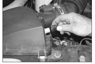
4. Disconnect the temp sensor electrical connection.
