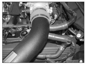
29. Reconnect the crankcase vent and idle air hose onto the new intake tube with the provided silicone hoses as shown.
