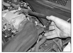
5. Disconnect the crankcase vent and idle air hoses as shown.
