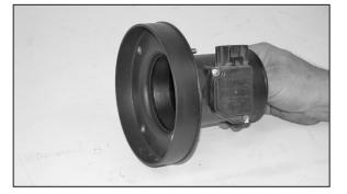
23. Assemble the filter adaptor onto the mass air sensor with the provided hardware as shown.
