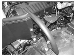
17. Install the saddle bracket assembly and the provided bracket (07093) onto the rubber mounted stud using the factory nut that was removed in step 8. onto vehicle as shown.
