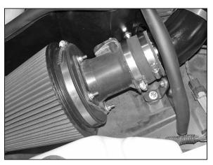
27. Install the mass air assembly onto the intake tube and adjust for best fit before tighting hose clamps.
