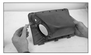
22. On vehicles that come equipped with an external temp sensor, twist counter clockwise to remove from air box lid.
