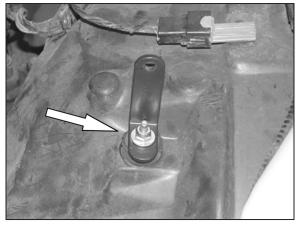
13. Install the provided bracket (07879) onto the inner wheel well as shown. NOTE: Install provided fender washer under wheel well when installing bracket.
