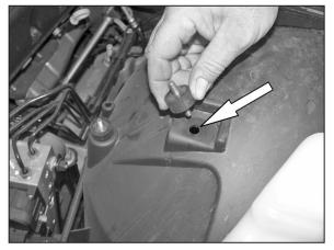
10. Remove the upper rubber mounted stud from the inner fender well as shown.
