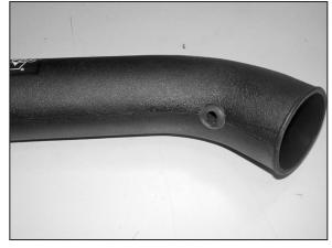
18. On vehicles that come with external temp sensor drill out the drill point with a 3/4 drill, then install the provided grommet as shown.
