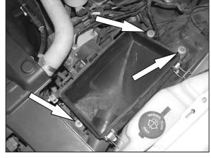
8. Remove the three 11mm bolts that retain the air box bottom to vehicle.
