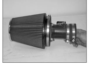
25. Install the air filter onto the mass air assembly as shown.
