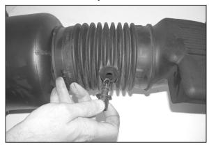
17. Remove the air temp. sensor from the stock air intake tube.
