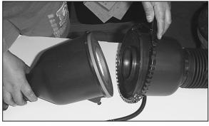
12. Open the air cleaner assembly and isolate the mass air sensor assembly.
