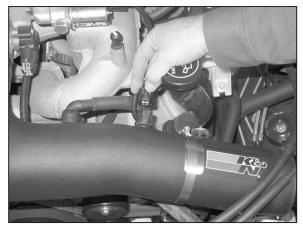
27. Reconnect the crank case valve vent, then reconnect the air temp sensor electrical connection
