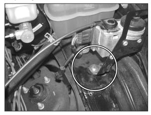
26. Install the provided rubber mounted stud under the cruise control bracket as shown.
