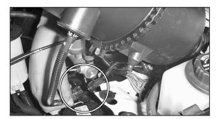
7. Disconnect the secondary mass air sensor electrical connection.
