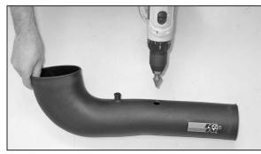
18. On vehicle's equipped with an external air temperature, drill a 5/8"id hole in the K&N® intake tube at the drill point as shown.
