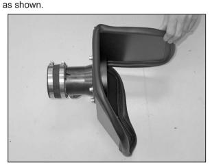
28. Install the silicone hose (08630) onto the mass air sensor.
