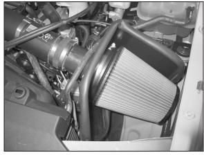
31. Install the K&N® air filter onto the mass air sensor assembly as shown.
