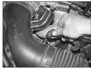
4. Remove the crank case valve hose from the stock intake tube.
