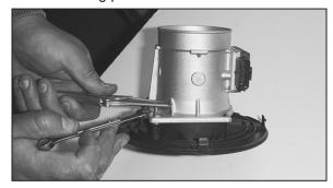
14. Using a pair of small vise grips or pliers, hold the stud while using a 10mm wrench to loosen the nuts, then remove the mass air sensor from the retaining plate.
