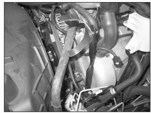
23. Install the saddle bracket assembly onto the valve cover stud with the provided hardware, then wire tie the wiring harness to bracket as shown.
