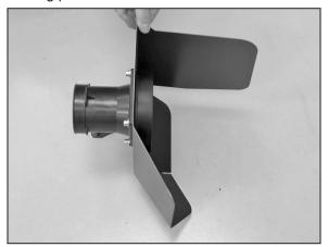
15. Assemble the heat shield and filter adapter onto the mass air sensor with the provided gaskets and hardware.
