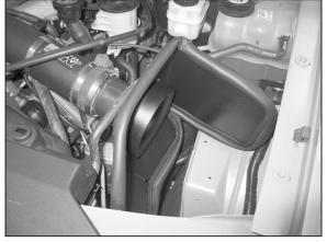
29. Install the mass air assembly onto the  $K\&N^{\otimes}$  intake tube as shown.
