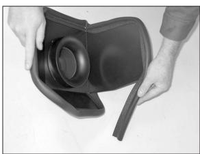
16. Install the edge trim onto the heat shield as shown. Trim if necessary.
