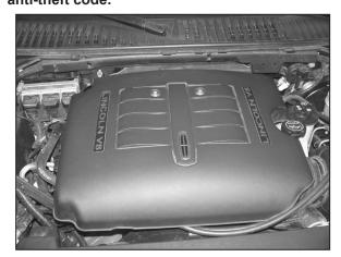
2. Loosen and remove two bolts that retain the engine cover, then remove cover.
