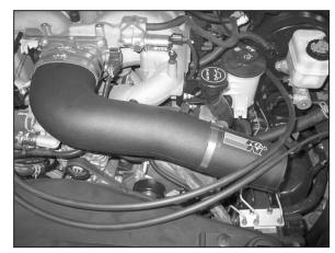
25. Install the new K&N® intake tube onto the throttle body and saddle bracket with the provided hose clamps.
