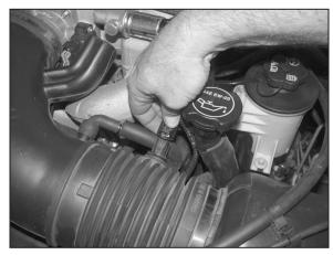
3. Disconnect the air temp sensor electrical connection.
