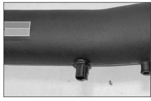
20. Install the air temp sensor into the grommet as shown.
