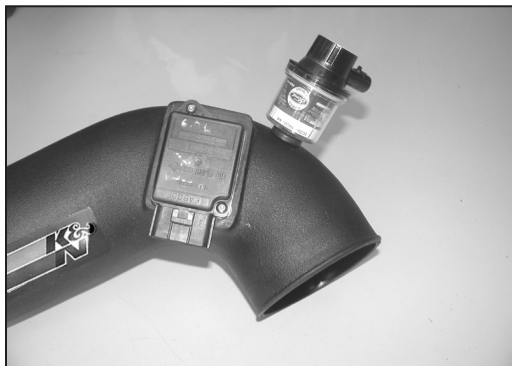
21. On vehicles equipped with a mass air sensor, install the mass air sensor into the K&N intake tube with the provided screws and spacers as shown.
