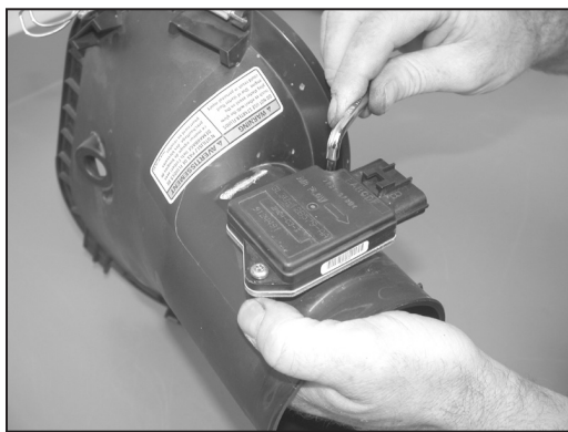
18. On vehicles equipped with a mass air sensor, remove the mass air sensor from the factory air box lid with the provided torx wrench as shown.
