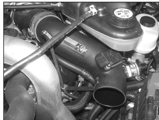
22. Install the K&N intake tube onto the turbo inlet with the provided hose clamp.
