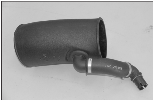
15d. On vehicles equipped with a one piece inlet tube and bellows, install the crank case vent tube assembly removed in step #15b into the grommet in the turbo inlet tube as shown.
