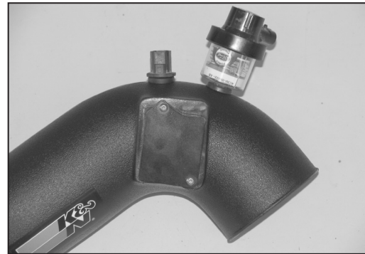
21d. On vehicles equipped with an air temperature sensor, install the factory grommet and air temperature sensor into the hole that was drilled in the previous step.
