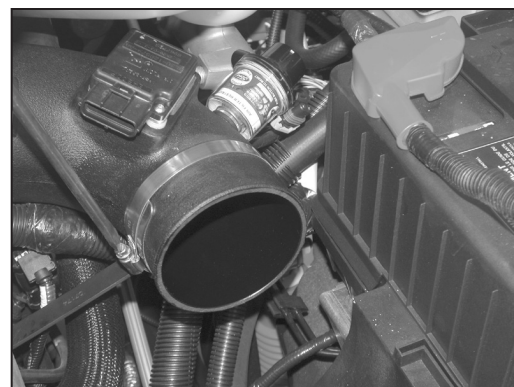
23. Secure the K&N intake tube to the saddle bracket with the provided hose clamp as shown.
