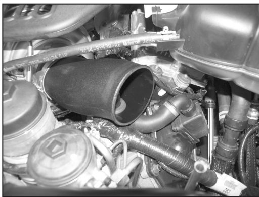
15e. On vehicles equipped with a one piece inlet tube and bellows, install the turbo inlet tube assembly onto the turbo. Rotate to align the crank case vent tube with the valve cover vent port. Snap the crank case vent tube into the valve cover vent port and secure the tube with the provided hose clamp.
