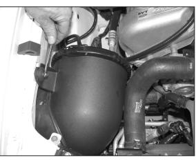
9. Loosen and remove the bolt that retains the air filter assembly onto the vehicle as shown.
