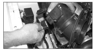
6. Disconnect the mass air electrial connection.
