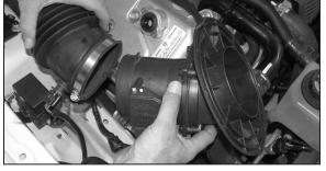
7. Disconnect the mass air from intake tube as shown.
