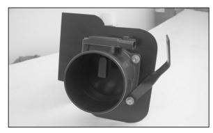
12. Install the provided bracket onto the mass air assembly with the 6mm x 25mm allen bolt as shown.
