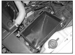
8. Remove the three nuts that retain the airbox bottom to vehicle.
