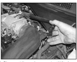
5. Disconnect the crank case vent and idle air hoses as shown.
