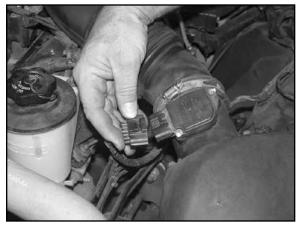
3. Disconnect the mass air sensor electrical connection.
