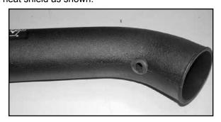
17. On vehicles that come with external temp sensor drill out the drill point with a 3/4 drill, then install the provided grommet as shown.
