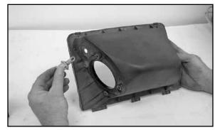
21. On vehicles that come equipped with an external temp sensor, twist counter clockwise to remove from airbox lid.
