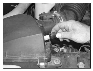
4. Disconnect the temp sensor electrical connection. Note: Not all vehicles come with external temp sensors.
