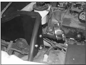
16. Install the saddle bracket assembly onto the heat shield as shown.
