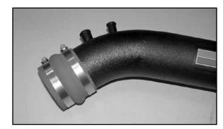
18. Install the provided silicone hump hose (087121) onto the K&N® intake tube with the provided hose clamps.
