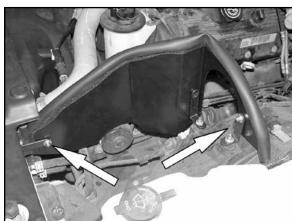
14. Install the heat shield into vehicle and attach to the two outter brackets.
