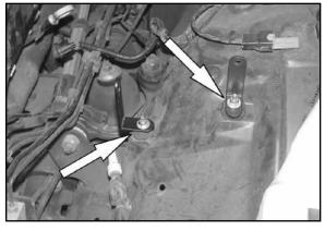
12. Install the two provided brackets onto the factory rubber mounted studs with the provided hardware.
