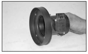
22. Assemble the filter adaptor onto the mass air sensor with the provided hardware as shown.
