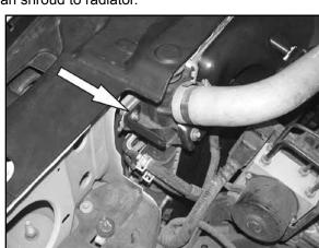
11. Install the provided bracket (07879) onto radiator with the provided hardware.
