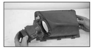
20. Remove the four bolts that retain the mass air sensor to the airbox lid, then remove the mass air sensor from lid.
