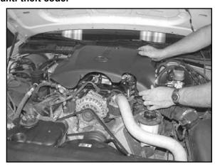
2. Loosen and remove the bolt that retains the engine cover to the engine with a 1/4 extension, then remove engine cover.
