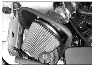
21. Install the heat shield assembly onto the K&N<sup>®</sup> intake tube and tighten the hose clamp as shown. **NOTE: Adjust heat shield for best clearance before tightening.**
