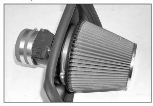
20. Install the K&N<sup>®</sup> air filter onto the heat shield assembly as shown.
