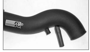
15. Install the silicone hose onto the K&N® intake tube as shown.
