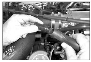
18. Remove the factory hose mender from vent hose as shown.
