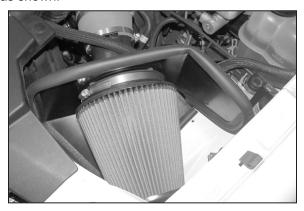
33. Install the K&N® Filtercharger onto the mass air assembly as shown.
