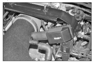
27. On 4.6L models, cut 1" off the provided 3/4" silicone hose. Then reconnect the resonator onto the intake tube as shown.
