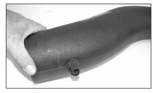
19. Install the air temp. sensor into the grommet as shown.
