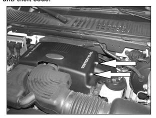
2. Loosen and remove the two bolts that retain the engine cover, then remove the cover.
