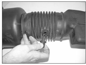
17. Remove the air temp. sensor from the stock air intake tube.
