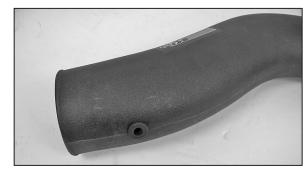
18. Install the provided grommet into the new intake tube as shown.
