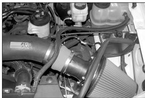
34. Disconnect the coolant return hose from the radiator and the reservoir, then swap ends and reconnect to radiator and reservoir.
