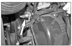
21. Remove the nut from stud as shown.
