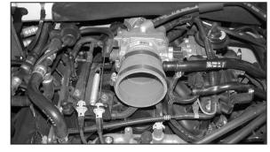
23. Install the silicone step hose (08724) onto the throttle body with the provided hose clamps.
