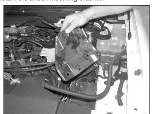
10. Remove the airbox mounting bracket from vehicle.
