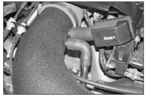
28. On 4.6L reconnect the crank case vent onto the intake tube as shown.
