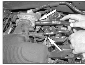
4. Remove the idle air control and the crankcase vent hose from the stock intake tube.
