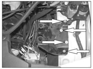
9. Using an 8mm socket, remove the 4 bolts that retain the airbox mounting bracket.
