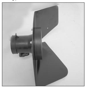
15. Assemble the heat shield and filter adapter onto the mass air sensor with the provided gaskets and hardware.
