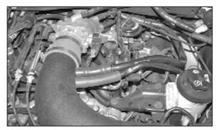
26. On 5.4L models install the idle air control and crankcase vent line onto the new intake tube with the provided silicone hose.
