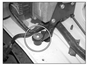
25. Install the provided rubber mounted stud under the cruise control bracket as shown.
