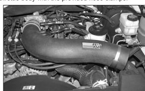
24. Install the new  $K\&N^{\otimes}$  intake tube onto the throttle body and saddle bracket with the provided hose clamps.
