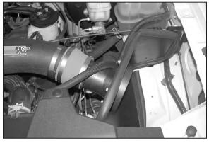
30. Install the mass air assembly onto the K&N® intake tube as shown.
