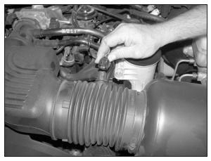
3. Disconnect the air temperature sensor electrical connection.
