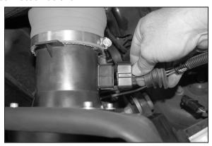
32. Reconnect the mass air electrical connection as shown.
