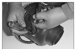
11. Slide the rubber grommet back and disconnect the primary mass air sensor electrical connection, using a flat blade screwdriver.
