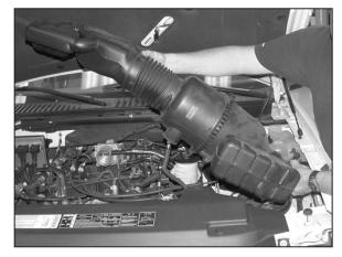
8. Remove the entire stock air intake assembly from the vehicle.
