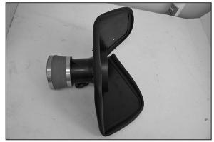
29 Install the silicone step hose (08050) onto the mass air sensor.
