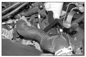
22. Install the saddle bracket assembly onto the stud with the provided hardware.
