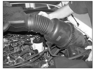
6. Detach the stock intake tube from the throttle body and lift up on the air cleaner assembly to release it from it's retaining grommets.
