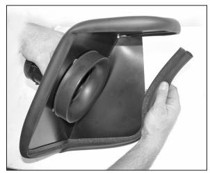
16. Install the edge trim onto the heat shield as shown. Trim if necessary.
