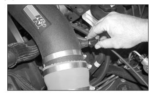
31. Reconnect the air temp sensor electrical connection as shown.
