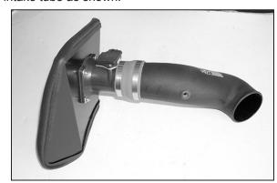
16. Install the rubber hose onto the K&N<sup>®</sup> intake tube as shown.
