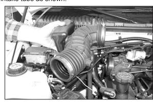
6. Loosen the hose clamp at the throttle body and at the mass air sensor, then remove the stock intake tube as shown.
