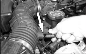
5. Remove the crankcase vent tube from the stock intake tube as shown.
