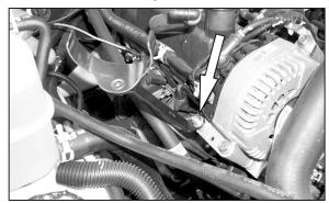
14. Install the saddle bracket assembly onto the alternator mounting stud with the provided 8mm nut and washer.
