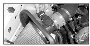
20. Re-connect the mass air sensor electrical connection as shown.
