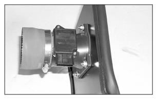
11. Assemble the silicone step hose (08051) and the hose clamps onto the heat shield assembly.
