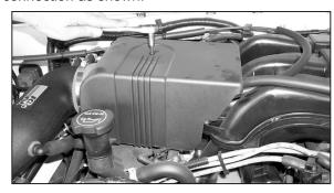
21. Re-install the throttle body cover with the two T25 torx screws that were removed in step #4.
