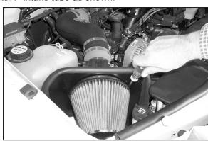
19. Install the K&N® Filtercharger onto the mass air adapter and secure it with the provided hose clamp.
