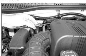
3. Release the cruise control cable from the intake tube as shown.
