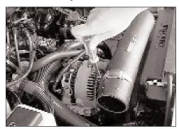
28. Using the provided hose clamp, secure the K&N® intake tube to the saddle bracket assembly as shown.
