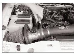
30. Install the heat shield assembly onto the K&N® intake tube and tighten the hose clamp as shown.
