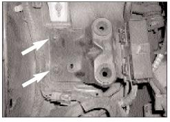
9. On vehicles that come equipped with relay switches mounted under airbox, remove the two bolts that retain the airbox mounting bracket.
