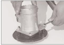
15. Loosen and remove the nuts from the mass air sensor.
