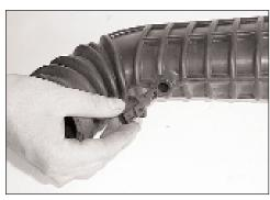
22. On models equipped with an external air temp. sensor, remove the air temp. sensor from the factory intake tube as shown.
