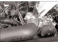
27. Install the K&N® intake tube onto the throttle body and secure as shown.
