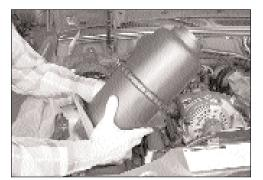
8. Pull firmly up on airbox to release airbox from grommets on the lower support bracket assembly.
