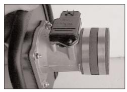
18. Install the silicone hose and hose clamps onto the heat shield assembly as shown.
