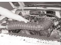
6. Loosen the hose clamps at the throttle body and at the airbox, then remove the air intake tube as shown.
