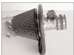
29. Install the K&N® Filter onto the heat shield assembly as shown.
