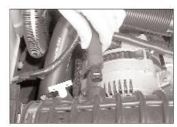
4. Remove the crankcase vent hose as shown.
