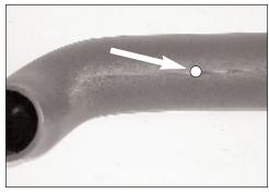
23. On models equipped with an external air temp sensor, drill out the drill point in the K&N® intake tube using a 11/16" drill bit.
