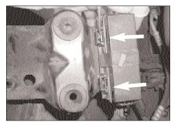
10. Use a flat blade screw driver to release clips then remove relays from bracket.
