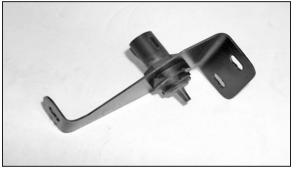
17. Using the stock retaining nut removed in step 16, secure the air temperature sensor to the air filter support bracket as shown.
