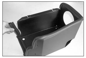
9. Apply the provided trim seal to the K&N<sup>®</sup> heat shield as shown.
