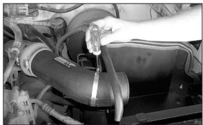
23. Secure the K&N<sup>®</sup> intake tube to the saddle bracket with the provided hose clamp as shown. **NOTE: Do not tighten completely as some adjustment may be necessary.**
