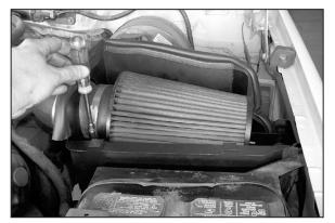
27. Tighten the hose clamp on the K&N<sup>®</sup> air filter as shown.
