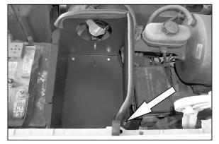
19. Install the K&N<sup>®</sup> heat shield assembly and push the rubber grommets onto the stock locating pins, then, secure the "L" bracket to the original air cleaner rubber mounting stud using the provided washer and nylock nut.
