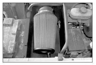
26. Install the K&N<sup>®</sup> air filter onto the K&N<sup>®</sup> intake tube, then, line up the stud on the filter with the air filter support bracket and secure with the provided hardware.
