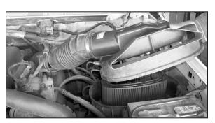
4. Loosen the hose clamp at the turbo inlet tube, then remove the upper air cleaner assembly as shown.
