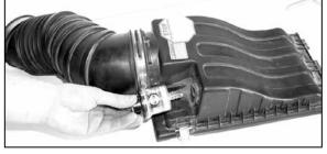
21. Remove air filter restriction gauge from stock airbox top.
