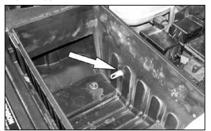
4. Remove the air temp sensor from the airbox.
