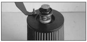
24. Install filter restriction gauge onto Air Filter top as shown.
