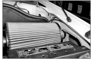
27. Adjust all brackets to obtain maximum clearance for intake tube and Air Filter element then tighten completely.
