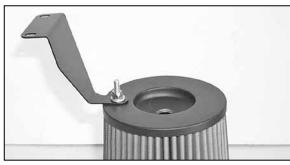
20. Install filter bracket onto filter as shown, but do not tighten completely.
