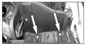
15. Using the two bolts removed in step 5, secure the heat shield to stock airbox mounting location. Do not tighten completely.
