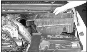
6. Then remove the stock airbox base from vehicle. NOTE: K&N Engineering, Inc., recommends that customers do not discard factory air intake.
