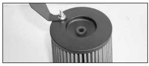
23. Install grommet into new Air Filter top as shown.
