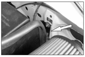
26. Now install the new filter bracket behind the fuse box mounting bracket as shown.
