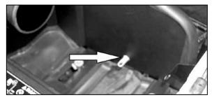
19. Install air temp sensor to heat shield as shown.
