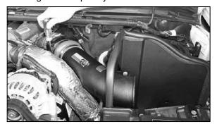
16. Install the K&N<sup>®</sup> intake tube onto intake manifold.
