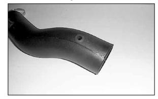
23. On models equipped with an external air temperature sensor, insert the grommet into the hole drilled in the K&N® intake tube.
