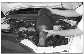
8. Pull upward firmly and remove the air cleaner.
