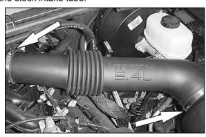
6. Loosen the hose clamps on the stock intake tube at the air cleaner and throttle body.
