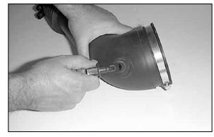
21. On models equipped with an external air temperature sensor, remove the air temperature sensor from the stock intake tube.
