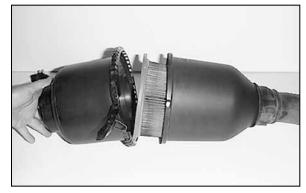
14. Disassemble the air cleaner assembly.
