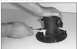
18. Loosen and remove the bolts that retain the mass air sensor to it's retaining plate.
