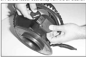
17. Disconnect the primary mass air sensor electrical connection.
