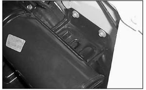
12. Loosen the two bolts that retain the evaporative canister mounting bracket to the inner fender.
