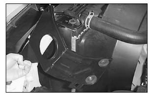
10. Remove the air cleaner mounting bracket. NOTE: On 2004 and later vehicles, this bracket is not removed as it is one piece.
