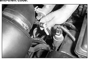
2. On models equipped with an external air temperature sensor, disconnect the air temperature sensor electrical connection.
