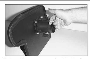
20. Assemble mass air sensor, heat shield and adapter using the gaskets and hardware provided.
