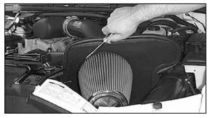
37. Install the air filter and tighten hose clamp.
