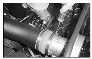
31. Tighten the hose clamp on the hump hose at the mass air sensor.
