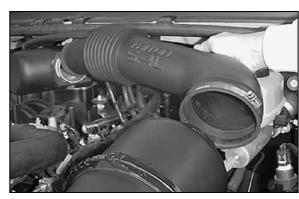
7. Remove the stock intake tube.
