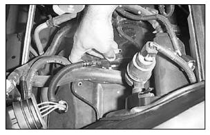
34. Reconnect the secondary mass air sensor electrical connection and reattach the wiring harness retaining clip to the inner fender apron.
