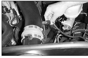
36. On models equipped with an external air temperature sensor, reconnect the air temperature sensor electrical connection and relocate the wiring harness retaining clip to front hole in the inner fender apron.
