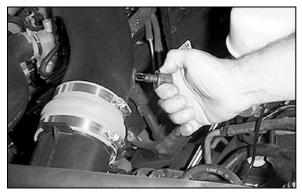
35. On models equipped with an external air temperature sensor, insert the air temperature sensor into the grommet in the intake tube.
