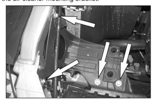
10a. On 2004 and later vehicles loosen and remove the four bolts, which retain the air box-evap canister bracket shown.
