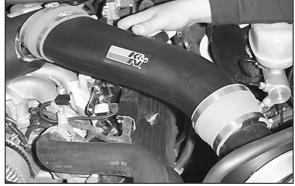
30. Install the intake tube.
