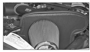
41. Install the Air Filter and tighten the hose clamp. NOTE: Drycharger® air filter wrap; part # RF-1020DK is available to purchase separately.
