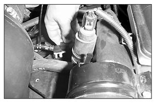
3. Detach the mass air sensor wiring harness from the inner fender apron.
