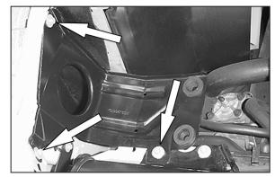
10. Loosen and remove the three bolts that retain the air cleaner mounting bracket.
