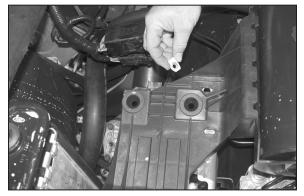
14a. On 2004 and later vehicles remove the clip nuts from under the air box-evap bracket as shown.
