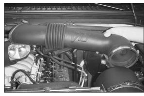
7. Remove the stock intake tube.
