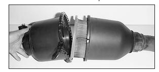
15. Disassemble the air cleaner assembly.
