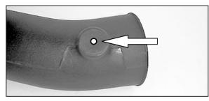
23. On models equipped with an external air temperature sensor, drill out the drill point in the K&N® intake tube using a 11/16" drill bit.
