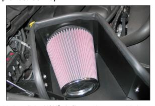
28. Install the  $K\&N^{\otimes}$  air filter and secure with the provided hose clamp.
