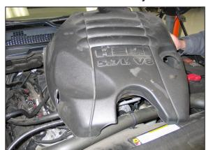
6. Lift up the engine cover to dislodge it from the mounting posts and then remove it from the vehicle.
