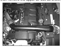
6. Loosen the two hose clamps that secure the intercooler transition tube. Then remove the intercooler transition tube.
