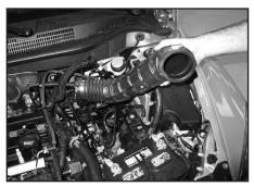
11. Loosen the hose clamp that secures the intake hose to the turbo inlet and then remove the intake tube from the vehicle.
