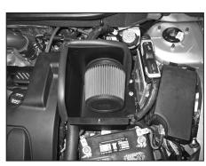
28. Install the K&N® <u>air filter</u> onto the intake tube and secure with the provided hose clamp.
