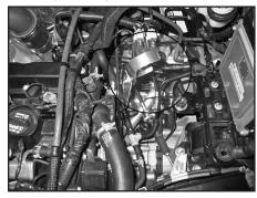
17. Secure the intake tube mounting bracket to the driver's side of the tab on the transmission using the provided hardware.
