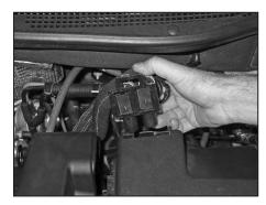
4. Release the clip which holds the vacuum switches to the upper air box and then unhook the vacuum switches from the air box.
