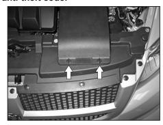
2. Unlock the two fresh air retaining clips by turning a 1/4 turn counter clockwise.
