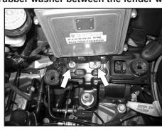
14. Remove the two ECU mounting nuts shown. **NOTE: These nuts will be reused in a later step.**
