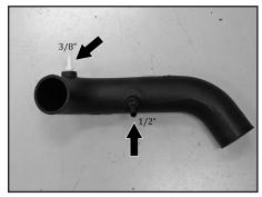
18. Install the two 1/4NPT fittings into the K&N® intake tube as shown.
