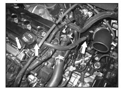
20. Install the provided crank case vent hose to the 1/4NPT X 1/2" on the K&N® intake tube and then attach the other end to the vent port on the valve cover as shown.
