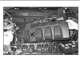
7. Lift up the engine cover to dislodge it from the mounting studs and then remove the engine cover
