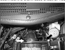
9. Loosen the hose clamp that secures the factory intake hose to the air box. Then unhook both the intake hose and vent hose from the air box.
