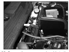
25. Secure the vacuum solenoids to the stud on the back of the heat shield using the provided hardware.
