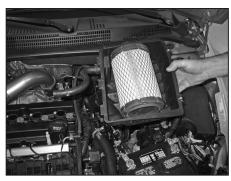
10. Lift up the air box to dislodge it from the mounting grommets. Then remove the air box from the vehicle.
