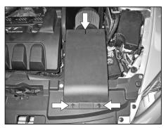
29. Install the fresh air intake duct onto the core support and heat shield, and then secure with the factory ¼ turn clips and hardware provided.
