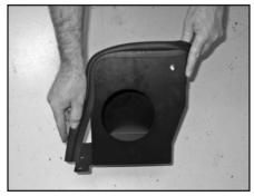
22. Install the provided edge trim onto the heat shield as shown.
