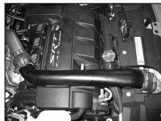
27. Reinstall the intercooler tube and secure with the factory hose clamps.
