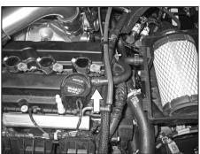
8. Release the spring clamp that secures the crank case breather hose to the valve cover. Then disconnect the crank case breather hose.
