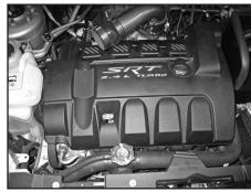
26. Reinstall the engine cover onto the valve cover.
