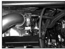
15. Install the provided silicone hose (08095) onto the turbo inlet and secure it with the provided hose clamp.
