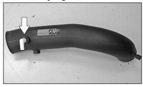
26. Install the 90°  $\frac{1}{4}$ " npt fitting into the intake tube as shown.
