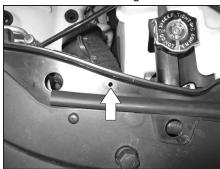
20. Drill a 1/4"O.D. hole at the marked location.
