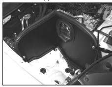
22. Install the heat shield assembly into the vehicle. Secure the rear of the heat shield to the mounting bracket installed onto the ECU. Secure the front heat shield mounting bracket to the radiator core support at the drilled location. Secure the bottom of the heat shield to the inner fender stud.
