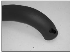
25. Install the air temperature sensor into the grommet installed into the intake tube as shown. NOTE: Handle the air temperature sensor with care as it is very fragile.
