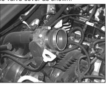
9. Install the silicone hose (084034) onto the throttle body and secure with the provided hose clamp.
