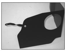
12. Secure the heat shield mounting bracket (070092) onto the heat shield as shown using the provided hardware.
