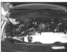
21. Remove the fresh air supply duct from the radiator core support as shown.
