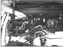
6. Remove the crank case vent tube assembly from the valve cover as shown.
