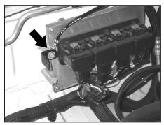
18. Install the heat shield mounting bracket (070066) onto the ECU and secure with the factory bolt removed in the previous step.
