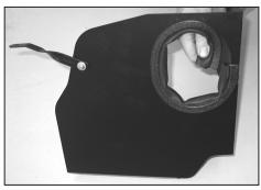
14. Install the provided edge trim into the hole of the heat shield as shown.
