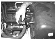
4. Disconnect the crank case vent hose from the air box as shown.
