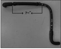
7. Using a knife, cut the crank case vent hose 7-1/2" from the valve cover elbow fitting as indicated.
