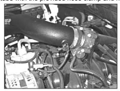
28. Reconnect the inlet air temperature sensor electrical connection.
