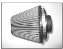
30. Install the filter adapter into the K&N <u>air filter</u> and secure with the provided hose clamp.
