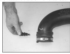
23. Remove the air temperature sensor from the factory intake tube as shown.
