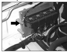
17. Remove the forward/upper ECU mounting bolt and ground strap.
