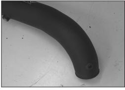
24. Install the supplied grommet into the intake tube as shown.
