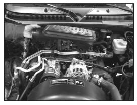
5. Lift to dislodge the intake plenum from it's mounting grommets and remove the intake plenum from the vehicle as shown.
