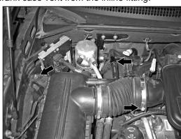
3. Disconnect the stock intake tube from the intake plenum. Lift to remove to remove the air box assembly from the vehicle as shown.
