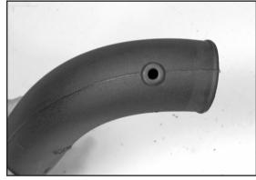
19. Install the provided grommet into the K&N<sup>®</sup> intake tube as shown.
