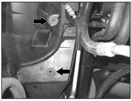
12. Install the two threaded inserts into the air box mounting grommets location as shown.
