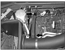
25. Install the provided silicone hose onto the 1/4npt fitting installed in the  $K\&N^{\circledR}$  intake tube and then attach the open end onto the hose to the factory crank case tube.
