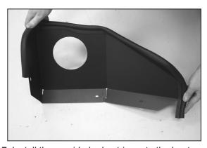
7. Install the provided edge trim onto the heat shield as shown.
