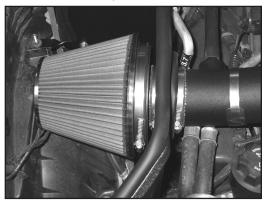
28. Install the <u>air filter</u> assembly onto the K&N<sup>®</sup> intake tube and secure with the provided hose clamp.
