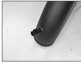
22. Install the air temperature sensor into the grommet installed into the K&N<sup>®</sup> intake tube in step #19.
