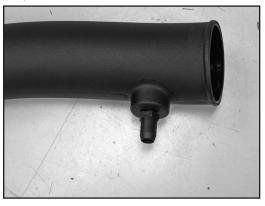
18. Install the provided  $\frac{1}{4}$  npt fitting into the K&N<sup>®</sup> intake tube as shown.
