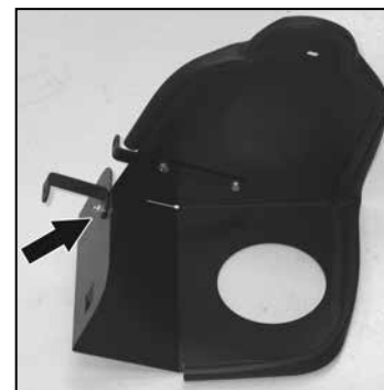
21. Install the heat shield mounting bracket (#070052) to the bottom of the heat shield using the provided hardware as shown.
