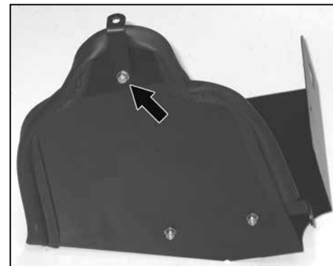
22. On 2007 model year vehicles, install the heat shield mounting bracket (#07805) to the side of the heat shield using the provided hardware. NOTE: The provided spacer is to be placed between the bracket and heat shield.
