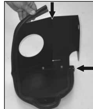
20. Install the provided edge trim onto the heat shield, starting at the bracket installed in step #19. NOTE: Some trimming of the edge trim may be necessary.
