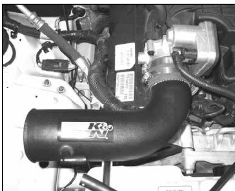
15. Install the K&N® intake tube into the silicone hose at the throttle body and align the mounting bracket with the timing cover bolt location (removed in step #8).
