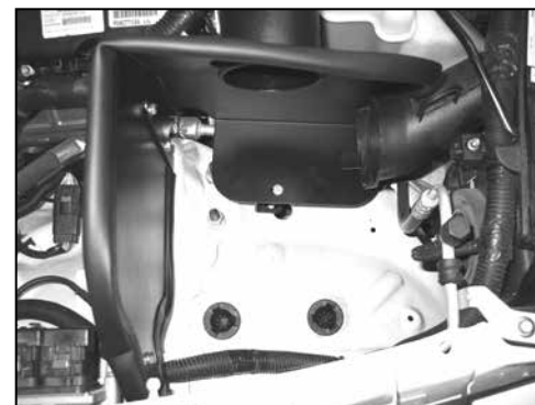
23. Install the heat shield into the engine compartment. Align the bottom rear mounting bracket with the threaded stud on the lower inner fender. Align the upper rear mounting bracket with the ECU mounting stud. Secure with the factory ECU mounting nut and provided hardware. NOTE: The fresh air duct must be aligned with the mounting tab on the bottom of the heat shield.
