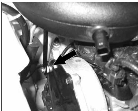
16. Secure the tube mounting bracket to the timing cover with the provided hardware as shown.
