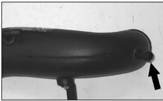
14. Install the air temperature sensor into the grommet installed into the K&N® intake tube as shown.
