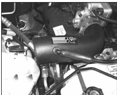
18. Connect the crank case vent hose to the 90° fitting installed into the K&N® intake tube as shown.
