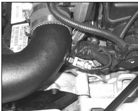
17. Re-connect the air temperature sensor electrical connection.
