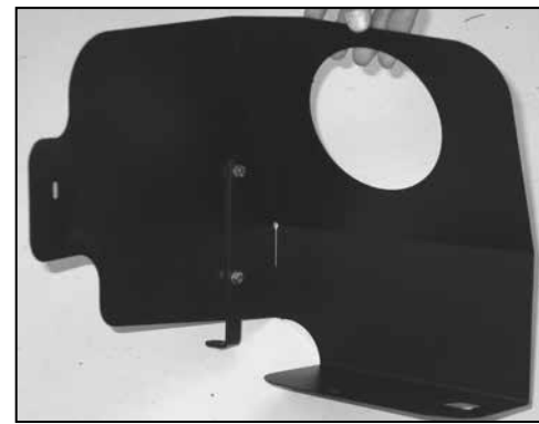
19. Install the heat shield mounting bracket (#07159) onto the heat shield using the provided hardware as shown.
