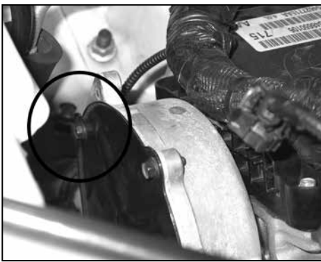
8. Remove the timing cover bolt (shown).
