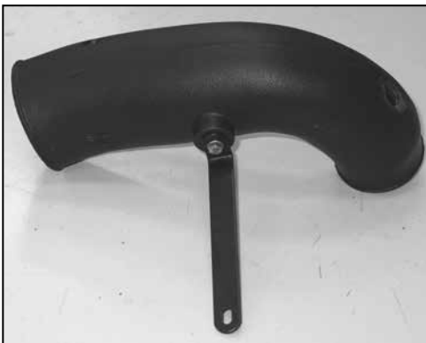
10. Install the tube mounting bracket (#06511) onto the K&N® intake tube (as shown) using the provided hardware.
