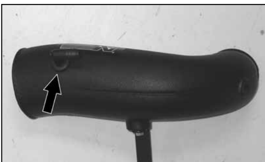
12. Install the provided 90° fitting into the grommet installed into the K&N® intake tube as shown. NOTE: On 2008 and later vehicles, it will be necessary to drill out the crank case vent hole to 7/8" id and install the larger grommet provided.
