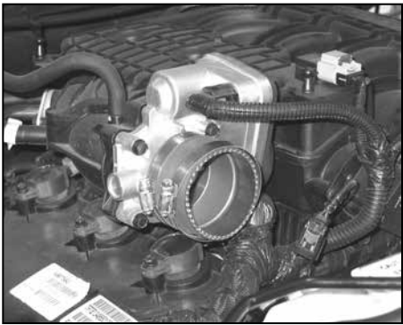
9. Install silicone hose (#08756) onto the throttle body and secure with the provided hose clamp.
