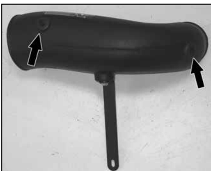
11. Install the provided grommets into the K&N® intake tube as shown.
