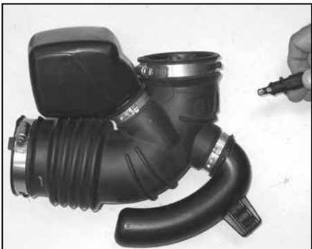
13. Remove the air temperature sensor from the stock intake tube as shown.
