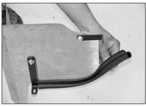
19. Install the short edge trim onto the heat shield assembly as shown.
