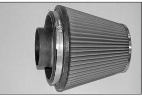
30. Install the air filter adapter into the K&N® air filter and secure with the provided hose clamp as shown.
