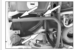
11. Lift the lower airbox, removing it from the vehicle as shown.
