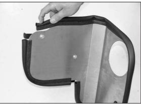
20. Install the long edge trim onto the heat shield assembly as shown.
