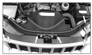
8. Remove the six grill retaining clips from the grille. Then, tilt the grille forward and lift, removing it from the vehicle.
