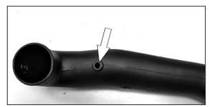
24. Install the provided grommet into the K&N® intake tube as shown.
