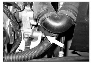
14. Remove the upper alternator mounting bolt as shown.
