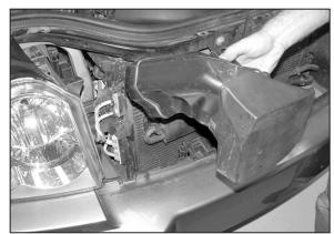
9. Pull the fresh air duct forward to disconnect it from the airbox, then remove it from the vehicle.
