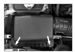
. Release the two airbox clam shell clips as
