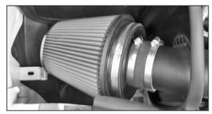
32. Install the K&N® air filter assembly onto the K&N® intake tube and secure with the provided hose clamp as shown.
