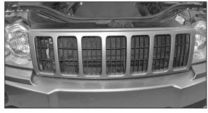
33. Re-install the grille assembly and secure with the factory retaining clips.
