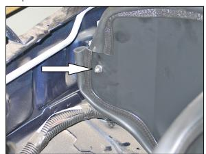
25a. On 2008 vehicles, secure the heat shield to the rubber mounted stud installed during step #21b.
