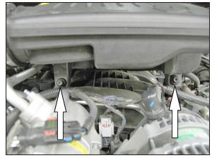
3. Remove the two "TORX" bolts that secure the intake plenum to the intake manifold with a T30 "TORX" wrench.
