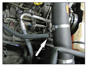
32. Install the provided silicone crankcase vent hose onto the fitting on the engine and then connect to the fitting on the intake tube.
