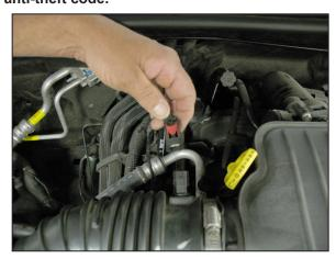
2. Release the red locking tab and then disconnect the air temperature electrical connection.
