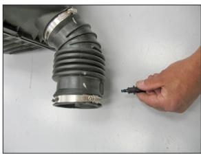
13. Remove the air temperature sensor from the stock intake tube.
