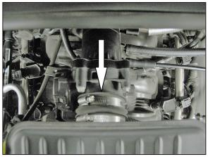
5. Loosen the hose clamp that secures the intake plenum to the throttle body.
