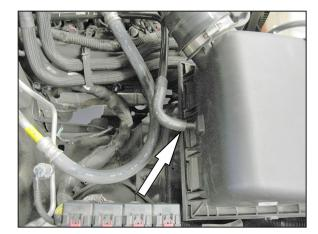
7. Disconnect the crankcase vent hose from the airbox.
