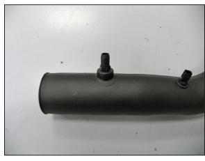
15. Install the provide ½"npt vent fitting into the intake tube as shown.
