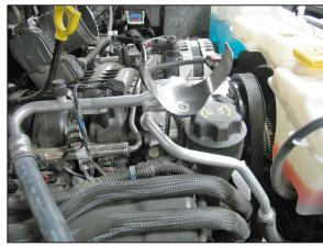
18. Install the tube mounting bracket assembly onto the A/C compressor and secure with the bolt removed in step #16.
