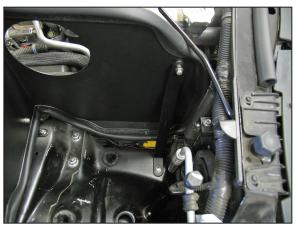
27. Secure the front heat shield mounting bracket to the inner fender with the hardware provided. NOTE: The bolt is to be installed from under the inner fender with the large fender washer through the factory hole in the inner fender and bracket.
