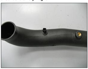
14. Install the air temperature sensor into the grommet installed in the intake tube during step #12.
