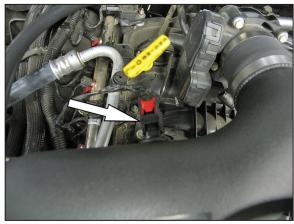
33. Reconnect the air temperature sensor electrical connection.
