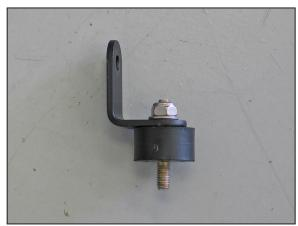
23a. On 2008 vehicles, attach the rubber mounted stud to the small "L" bracket (070066) with the provided hardware as shown.
