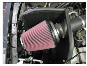
31. Install the filter assembly onto the intake tube and secure with the provided hose clamp.
