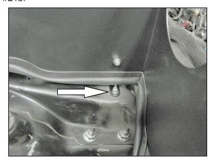
26. Secure the lower heat shield mounting bracket to the stud on the inner fender with the hardware provided.
