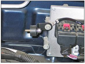
23b. On 2008 vehicles, attach the "L" bracket assembly from step #21a. to the ECU using the factory bolt removed in step #11a.
