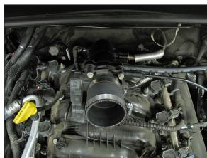
19. Install the silicone hose (08096) onto the throttle body and secure with the provided hose clamp.
