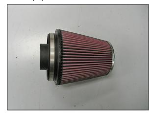
29. Install the filter adapter into the K&N® air filter and secure with the provided hose clamp.
