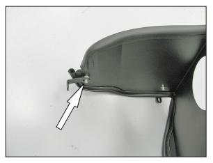
23. On 2007 vehicles, install the remaining small "L" bracket (06464) onto the heat shield with the provided spacer and hardware.
