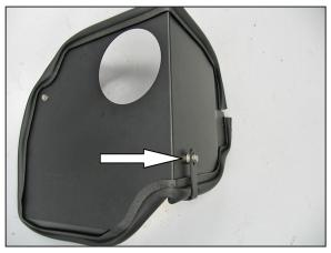
22. Install the small "L" bracket (070742) onto the heat shield as shown using the spacer and hardware provided.
