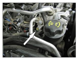
16. Remove the A/C compressor mounting bolt shown.
