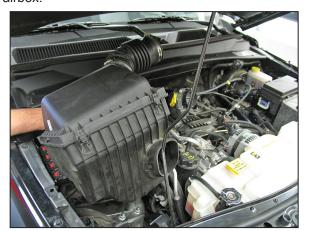
8. Pull up on the airbox assembly to dislodge it from the mounting grommets and then remove the airbox assembly from the vehicle.
