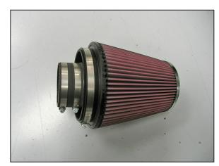
30. Install the silicone hose (08630) onto the air filter adapter and secure with the provided hose clamp.
