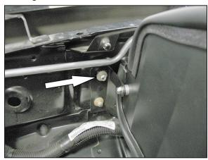
25. On 2007 model year vehicles, secure the upper heat shield mounting bracket with the nut removed in step #11.
