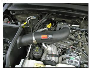
28. Install the intake tube into the silicone hose at the throttle body and align with the mounting bracket installed in step #17. Secure the tube with hose clamps provided.
