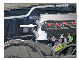
11a. On 2008 vehicles, remove the front-upper ECU mounting bolt shown.
