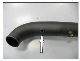
12. Install the provided grommet into the intake tube as shown.
