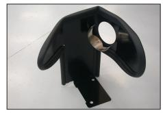
12. Install the saddle bracket assembly onto the heat shield as shown using the provided hardware.
