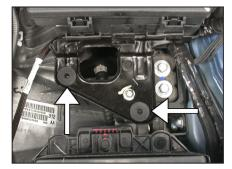
13. Install the two provided inserted nuts into the airbox mounting plate as shown.
