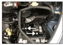
14. Install the heat shield onto the inserted nuts installed in step #13 and secure with the provided bolts and washers.
