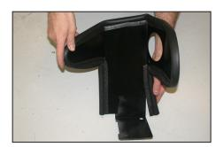
10. Install the short edge trim onto the heat shield as shown.
