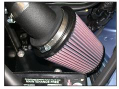
22. Install the K&N<sup>®</sup> filter assembly onto the K&N<sup>®</sup> intake tube, adjust the intake kit for the best fit and tighten all of the hose clamps. NOTE: Drycharger<sup>®</sup> air filter wrap; part # RP-4660DK is available to purchase separately.
