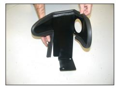
9. Install the long edge trim onto the heat shield as shown.
