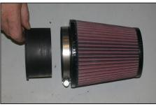
21. Install the provided filter adapter into the  $K\&N^{\circledast}$  air filter as shown.
