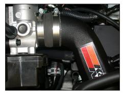
19. Connect the provided crankcase vent hose onto the valve cover and then the K&N $^{\odot}$  intake tube as shown.
