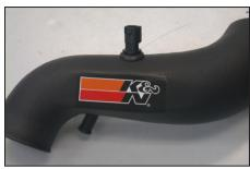
17. Install the air temperature sensor into the  $K\&N^{\otimes}$  intake tube as shown.
