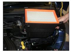
6. Pull up firmly on the airbox base to dislodge it from the retaining grommets and then remove the airbox from the vehicle.
