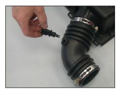
16. Carefully remove the air temperature sensor from the stock intake tube as shown. **NOTE: Use care when removing the sensor as it is very fragile.**
