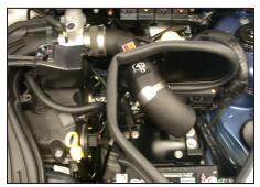
18. Feed the K&N<sup>®</sup> intake tube through the heat shield and saddle clamp and then into the silicone hose at the throttle body. Do not completely tighten at this time.
