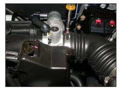
3. Loosen the hose clamp, which secures the intake tube to the throttle body.
