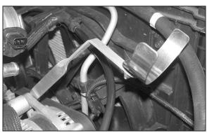
18. Install the saddle bracket assembly onto the alternator with bolt removed in step 17.
