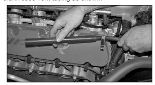
37. Install the supplied silicone vent hose onto the factory crank case vent tubing as shown.
