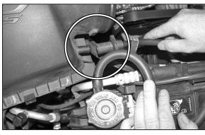
5. Loosen the crankcase vent tube clamp, and then disconnect the vent tube from the air box lid as shown.
