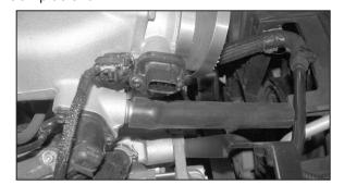
29. Install the provided silicone hose onto the idle air vent port as shown.
