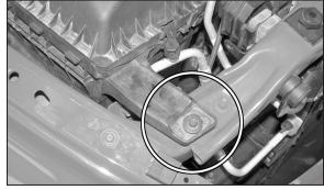
6. Remove the air box mounting nut shown.
