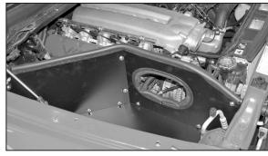
25. Install the heat shield assembly into the vehicle and secure to the mounting brackets installed in steps #23 and #24 with the provided hardware.
