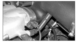
34. Install the idle air hose onto the K&N® intake tube as shown.
