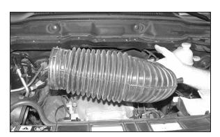
4. Loosen the two hose clamps that secure the intake tube to the throttle body and factory air box, and then remove the intake tube from the vehicle.
