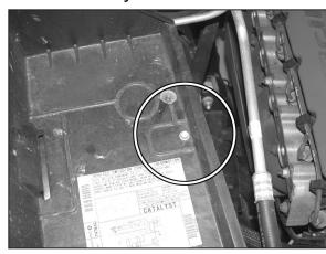
8. Remove the heater hose bracket mounting bolt shown.
