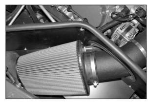
40. Install the K&N® air filter onto the K&N® intake tube as shown; the base of the filter flange should meet the 2nd bead on the intake tube. Line up the hose mender with the crankcase vent hose and then install the vent hose onto the hose mender. Secure the filter with the provided hose clamp. NOTE: Rotate the filter on the intake tube to obtain minimum of 1/2" clearance of the filter material to the heat shield.
