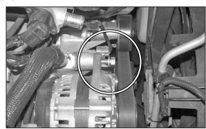
17. Remove the upper alternator mounting bolt as shown.
