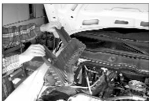
12. Remove the air box mount as shown.
