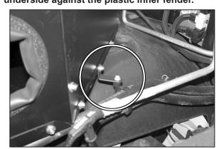
27. Using the bolt removed in step #8, secure the heater hose-mounting bracket to the "L" bracket installed on the heat shield in step #19.
