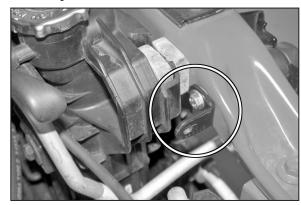
23. Install the "L" bracket (070066) onto the radiator core support with the provided hardware as shown.
