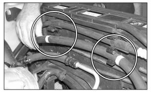
14. Unhook the A/C hose from the mounting clips on the radiator fan shroud as shown.
