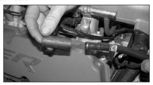
36. Remove the rubber coupling hose from the crank case vent tubing as shown.
