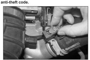
2. Depress the locking tab and then disconnect air temperature sensor electrical connection as shown.
