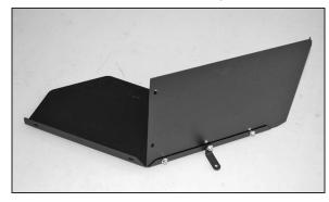
19. Install the heat shield side panel (074031) onto the heat shield base (074030) with the "L" bracket (07078) as shown with the provided hardware. NOTE: The L bracket should be installed at the center mounting location with the 16mm long bolt. Do not completely tighten the bolts at this time.
