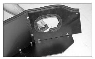
22. Install the provided edge trim into the hole in the heat shield as shown.
