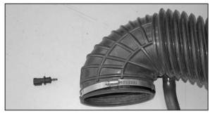
31. Remove the air temperature sensor from the stock intake tube as shown.
