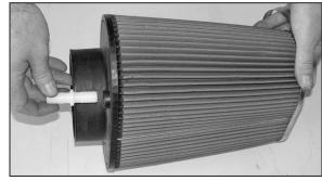
39. Install the supplied hose mender into the K&N® air filter as shown.
