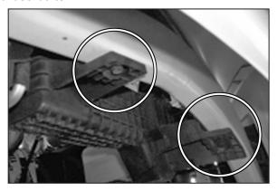
10. Use a 13mm wrench to remove the two bolts that retain the lower airbox mount.
