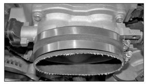
28. Install the silicone hose (08623) onto the throttle body and secure with the provided hose clamp as shown.
