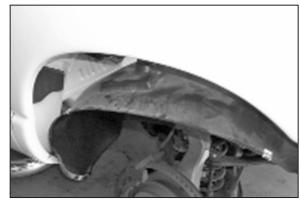
9. Remove the 8 bolts that retain the inner fender to the vehicle. To allow inner fender wall to drop for access to the lower airbox mount bolts.
