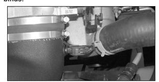
35. Reconnect the air temperature electrical connection.
