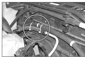
15. Using the tie-wraps provided, strap the A/C hose to the P/S hose as shown.
