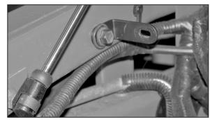
24. Install the "L" bracket (070712) onto the inner fender with one of the bolts removed in step #11.
