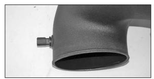
32. Install the air temperature sensor into the grommet installed into the K&N® intake tube as shown.
