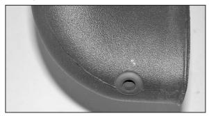
30. Install the provided grommet into the K&N® intake tube as shown.
