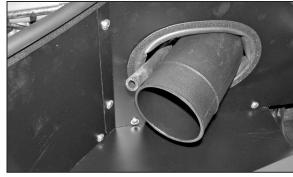
38. Pass the new crank case vent hose through the heat shield as shown.
