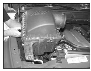
7. Remove the air box assembly from the vehicle as shown.
