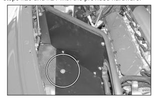
26. Install the heat shield mounting bolt through the base of the heat shield and through the inner fender well, secure with the provided nut.
