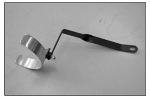
16. Assemble the saddle bracket assembly as shown.
