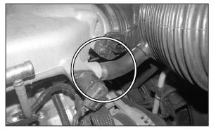
3. Remove the idle air hose from the idle air solenoid as shown.
