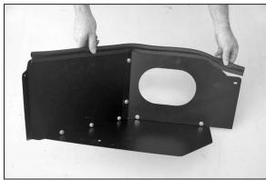
21. Install the provided edge trim onto the heat shield as shown.
