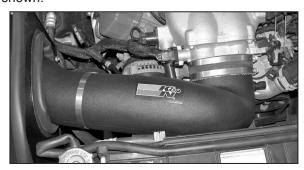
33. Install the K&N® <u>intake tube</u> into the silicone hose on the throttle body and onto the saddle clamp then secure with the provided hose clamps as shown.
