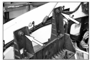
11. Use a 13mm wrench to remove the two bolts that retain the upper airbox mount.
