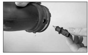
20. Remove the air temperature sensor from the stock intake tube as shown.
