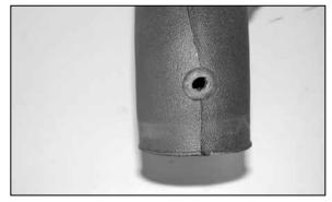
19. Install the provided grommet in the  $K\&N^{\ensuremath{\$}}$  intake tube as shown.
