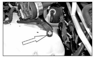
14. Install the provided 1/4 washer onto existing nut that retains the cruise control bracket to vehicle.
