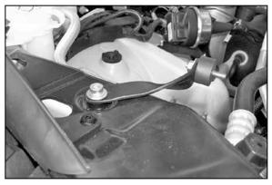
12. Install the bracket onto core support with the provided hardware as shown.
