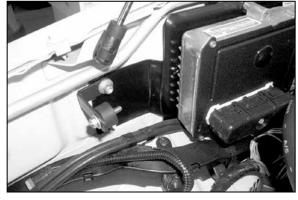
8. Secure "L" bracket to inner fender with the nut that was removed in the previous step.
