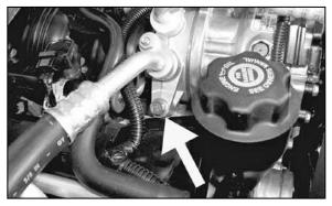
17. Remove the A/C compressor-mounting bolt.
