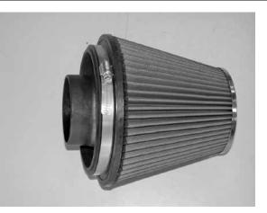
28. Install the filter adapter into the air filter as shown, secure with the provided hose clamp.
