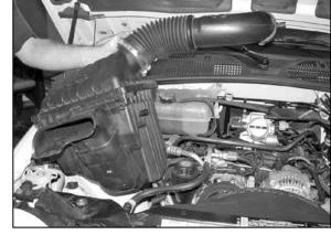
5. Firmly lift up to disengage the airbox from the retaining grommets and remove the airbox from the vehicle.
