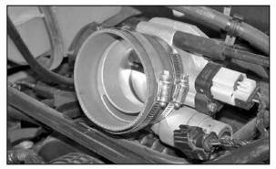
18. On 2006 and earlier vehicles, install the provided silicone hose (08690) onto the throttle body with the provided hose clamps as shown.
