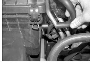
4. Disconnect the stock crankcase vent hose from the airbox as shown.
