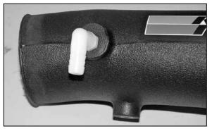
22. Install the 90° NPT fitting into the K&N $^{\mbox{\tiny \$}}$  intake tube as shown.
