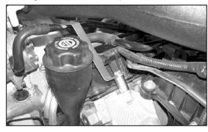
24. On vehicles not equipped with A/C, use the spacer and bolt provided to secure the mounting bracket to the engine.
