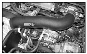
23. Install the K&N<sup>®</sup> intake tube into the silicone hose at throttle body, position the tube mounting bracket to line up on the A/C pump with the bolt removed in step #17. Then secure bracket to intake tube with the provided hardware. Then tighten the hose clamp at the throttle body and the AC mounting bolt removed in step #17.
