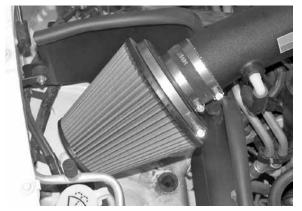
30. Install the air filter assembly onto the K&N<sup>®</sup> intake tube as shown and secure with the provided hose clamp.
