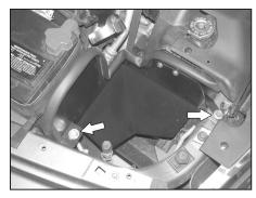
16. Install the K&N® heat shield assembly and secure the mounting bracket to the radiator core support with original bolt removed in step #13. Secure the rear of the heat shield to the 3/8" threaded insert with the provided hardware.
