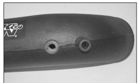
20. Install the provided grommet into the K&N<sup>®</sup> intake tube as shown.
