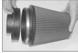
26. Install the provided radiuses filter adapter into the K&N<sup>®</sup> air filter and secure with the provided hose clamp.
