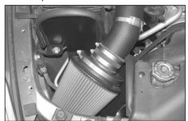
28. Install the K&N® air filter assembly onto the K&N® intake tube and secure with the provided hose clamp.
