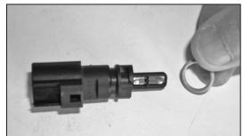
19. Remove the O-ring from the air temp sensor as shown.
