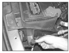
15. Install the 3/8" threaded insert provided into the air box mounting grommet hole vacated in step #14.
