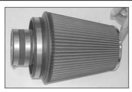
27. Install the silicone hose (08630) onto the K&N<sup>®</sup> air filter assembly and secure with the provided hose clamp.
