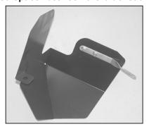
12. Install the heat shield bracket (07197) onto the heat shield with the provided hardware.
