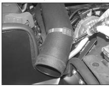
23. Using the provided hose clamp, secure the  $K\&N^{\otimes}$  intake tube to the saddle bracket assembly as shown.
