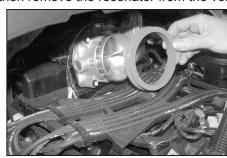
9. Remove the resonator silicone gasket from the throttle body.
