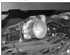
17. Install the silicone hose (08630) onto the throttle body and secure with the provided hose clamp.
