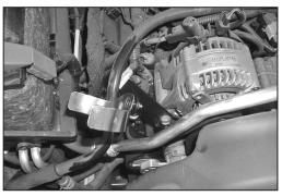
11a. On 2008 and later model year vehicles, attach the tube mounting bracket assembly (070101) to the alternator mounting bolt as shown.
