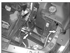
14. Remove the core support mounting bolt shown with a 13mm wrench, and pull out the stock air box mounting grommet shown.
