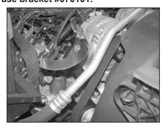
11. On 2007 and earlier model vehicles, install the tube bracket assembly as shown using the hardware provided.
