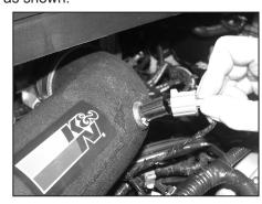
24. Reconnect the temp sensor electrical connection.
