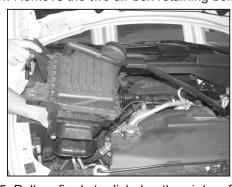
5. Pull up firmly to dislodge the air box from the mounting grommet, and remove the air box from the vehicle.
