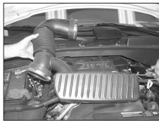
3. Loosen the intake tube hose clamps and remove the intake tube assembly from the vehicle.
