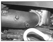
22. Install the intake tube onto the throttle body and secure with the provided hose clamp.
