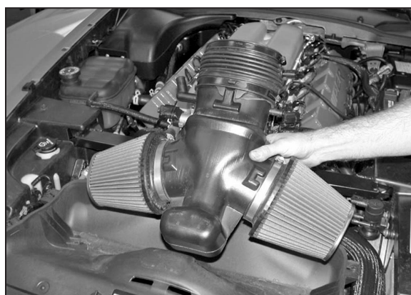
5. Loosen intake tube hose clamp at throttle body, and remove wing nut under tube. Then remove complete intake assembly. NOTE: K&N Engineering, Inc., recommends that customers do not discard factory air intake.
