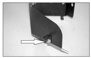
22. Install the provided bracket (070066) onto heat shield with the provided hardware as shown. Do not tighten completely
