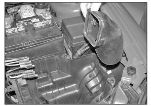
2. Release the two clips that secure the wiring harness to air box as shown.
