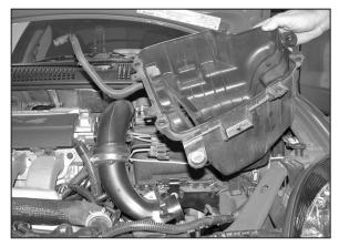
10. Remove the two 10mm bolts that secure the air box to vehicle, then remove air box from vehicle as shown.
