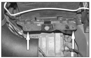
26. Remove the two 10mm bolts from battery tray as shown.
