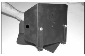
20. Install the provided brackets (070952) onto heat shield with the provided hardware as shown. Do not tighten completely.
