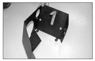
21. Install the provided bracket (071001) onto heat shield with the provided hardware as shown. **NOTE: The holes that are off set, do not mount to heat shield.**
