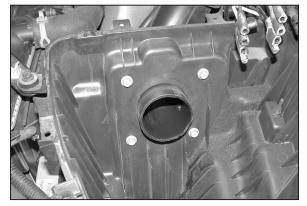
6. Remove the four 10mm bolt that secure the intake tube to air box.
