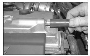
17. Install the provided silicone hose onto the valve cover as shown.
