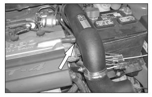
18. Install the K&N<sup>®</sup> intake tube onto the turbo, then align with saddle bracket. Then tighten all hose clamps.
