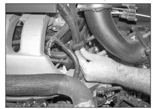
11. Remove the intake vent line from intake tube as shown.
