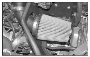
32. Install the K&N<sup>®</sup> filter charger onto the filter adapter as shown.
