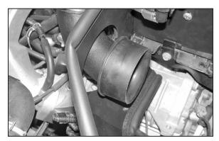
31. Install the filter adapter onto the new K&N<sup>®</sup> intake tube as shown.
