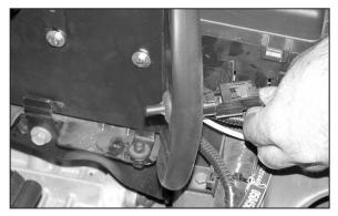
30. Install temp sensor into heat shield then reconnect the electrical connection as shown.
