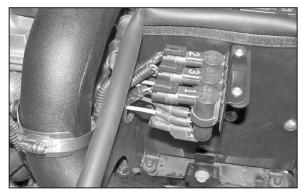
28. Connect the solenoid pack onto heat shield with the provided hardware, then reconnect the vacuum lines and electrical connections onto solenoid as shown.
