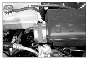
17. Install the provided silicone hose onto the resonator with the provided hose clamps as shown.
