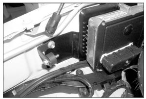
5a. Secure "L" bracket to inner fender with the nut that was removed in the previous step.
