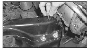
11a. Vehicles that do not come equipped with cruise control, install the provided spacer and washer onto the stud as shown.
