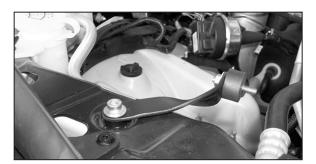
9. Install the bracket onto core support with the provided allen bolt as shown.
