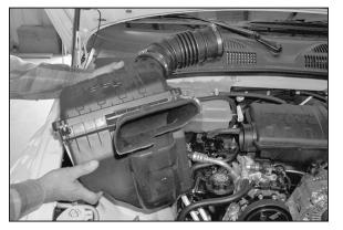
3. Firmly lift up to disengage air box from retaining grommets and remove air box from vehicle. NOTE: K&N Engineering, Inc., recommends that customers do not discard factory air intake.
