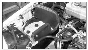
12. Install heat shield onto the vehicle with the provided hardware as shown.
