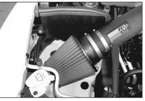
19. Install the K&N<sup>®</sup> Filtercharger onto the new K&N<sup>®</sup> intake tube as shown. NOTE: Drycharger<sup>®</sup> air filter wrap; part # RC-5060DK is available to purchase separately.
