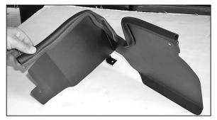
10. Install edge trim onto heat shield as shown. Trim if needed.
