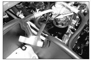
15. Install the "Z" bracket onto the A/C compressor and secure with the bolt that was removed in step 13.
