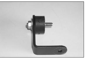
4. Assemble "L" bracket and rubber mounted stud as shown.
