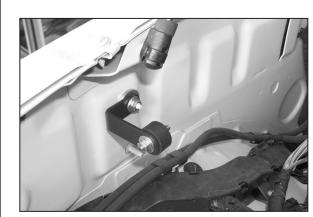
6. Mount "L" bracket onto existing stud with the provided hardware.
