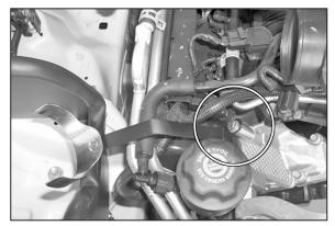
16. On vehicles that do not come equipped with A/C, mount the "Z" bracket onto the intake manifold with the provided hardware.
