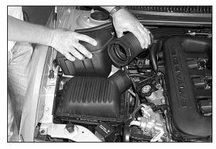
4. By pulling upward, remove Center Intake Tract Assembly off the grommet.
