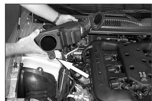
8. Lubricate Grommet and remove rear Intake tract Assembly.
