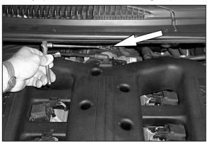
7. Loosen Hose Clamp at the Throttle Body using a 1/4" socket.
