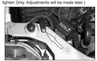
20. Install small Heat Shield Bracket on hole located behind the passenger-side headlight, using a 6mm Bolt, (2) Flat Washers, and a Lock Nut. (Hand tighten Only. Adjustments will be made later.)
