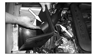
22. Place Intake Tube through hole of Heat Shield, and insert 1" tapered, Pin Boss (see #13) over Locating Pin, as shown.
