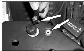
19. Place the white, nylon Spacer, as shown, and install the Heat Shield Bracket on hole located behind the passenger-side headlight, using a 6mm Bolt, (2) Flat Washers, and a Lock Nut.. (Hand tighter Only Adjustments will be made letter)
