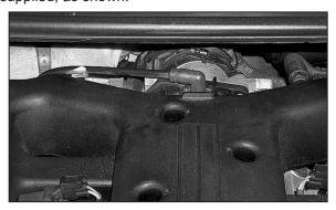
11. Reinstall Throttle Body Hose to throttle body and tighten Hose Clamp.
