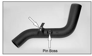
13. Clean the inside of the K&N® Intake Tube and assemble Bracket to Intake Tube using (2) Bolts and (2) Wave Washers. (Hand tighten only.)
