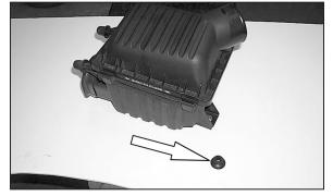
15. Remove Grommet from Airbox, as shown.
