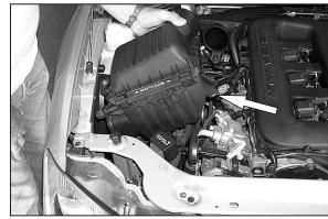
5. Lubricate Grommet and remove Front Airbox in an upward direction.
