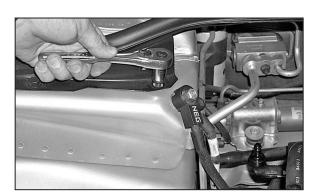
14. Remove Cowl Bolt located above the Negative Battery Cable, using a 3/8" Drive Ratchet and a 13mm socket. (Bolt will be reused.)
