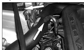
26. Tighten Heat Shield Bracket Bolts and Cowl Bolt. Install Vent Hose to Intake Tube, as shown.
