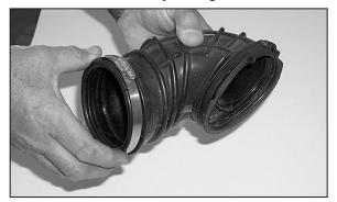
10. Replace Metal Band with #56 Hose Clamp supplied, as shown.
