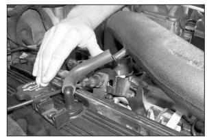
19. Install the 5 inch hose onto the crankcase vent, then connect the other end to the vent on the K&N^ $^{\odot}$  intake tube as shown
