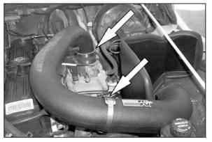
17. Install the K&N<sup>®</sup> intake tube into the silicone hose and line up the other end of the tube with the saddle bracket, then secure the tube to the throttle body and the saddle bracket with the provided hose clamp
