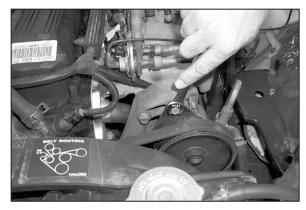
7. Remove the upper power steering pivot bolt as shown
