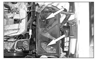
6. Loosen and remove the two bolts that secure the lower air cleaner assembly, then remove lower airbox from vehicle.
