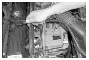
2. Disconnect the crank case vent hose.
