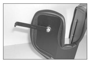
10. Install small "L" bracket onto the heat shield as shown
