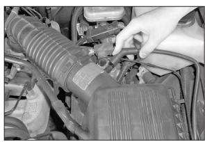
3. Remove the EVAP canister vent line from the air intake tube.
