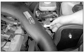
17. Install the 1/4 x 3/8" vent fitting onto the K&N® intake tube as shown.
