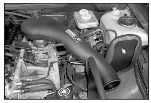
15. Install the K&N® intake tube onto the throttle body then tighten the hose clamp.
