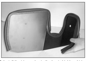
7. Install the trim seal onto the heat shield and trim if necessary.
