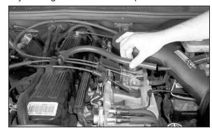
16. Install the provided silicone hose onto the crankcase vent on the valve cover, then install the other end onto the K&N® intake tube.
