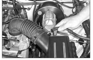
3. Remove the EVAP canister vent line from the air cleaner lid.
