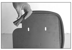
7. Install the trim seal onto the heat shield. Trim excess if needed
