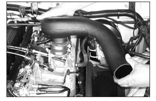
13. Install the K&N<sup>®</sup> <u>intake tube</u> onto the throttle body and tighten the hose clamp.
