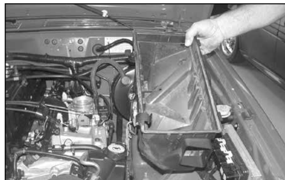
5. Loosen and remove the two bolts, and one nut to remove the lower air box assembly. NOTE: K&N Engineering, Inc., recommends that customers do not discard factory air intake.
