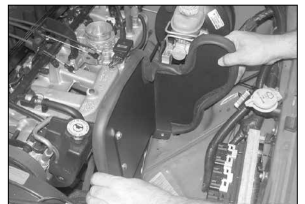
8. Install the heat shield into the vehicle as shown.
