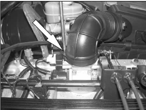
2. Loosen the hose clamp at the throttle body.
