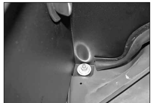
9. Secure the heat shield to the original air box mounting stud using the provided washers, and the nut removed in step 5. Do not tighten completely.
