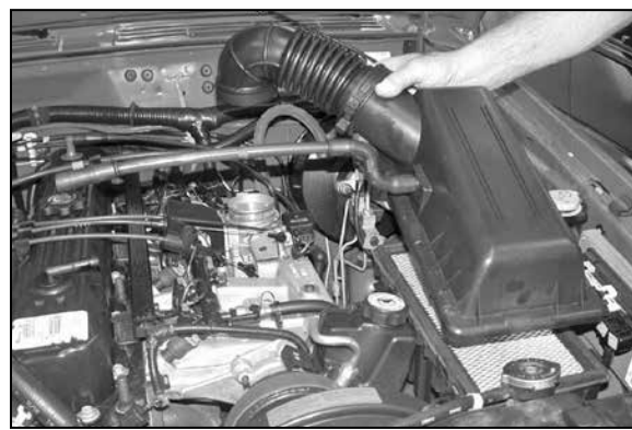
4. Unclip the air box lid, then, remove the upper intake assembly.
