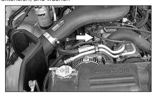
35. Secure the saddle bracket to the K&N<sup>®</sup> intake tube with the provided hose clamp as shown, then tighten the bolt at the fuel rail (see arrow). Position the heat shield for best fit and clearance.
