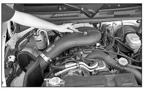
34. Install the K&N® intake tube onto the throttle body and secure the plenum with the provided nut extension, and washer.
