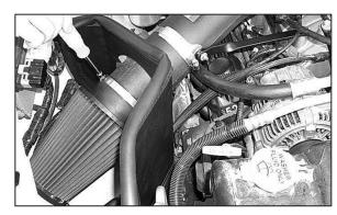
37. Install the  $K\&N^{\otimes}$  Air Filter and secure with the provided hose clamp.
