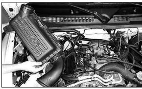
4. Loosen and remove the nut that secures the air box to the inner fender, then pull firmly upward to release the air box from its mounting grommets and remove the air box assembly.
