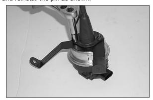
16. Using the original nuts secure the cover to the cruise control assembly, as shown.
