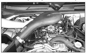
33. Slide the K&N<sup>®</sup> intake tube through the hole in the heat shield as shown.
