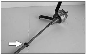
17. Slide the provided grommet over the cable ends as shown.
