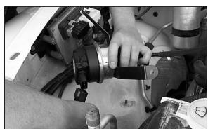
18. Position the cruise control into the vehicle in order to reconnect the cruise control electrical connection as shown.
