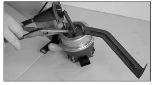
13. Loosen and remove the two nuts that secure the cruise control actuator to the bracket, then slide the diaphragm cover upwards and remove the pin from the cable end.
