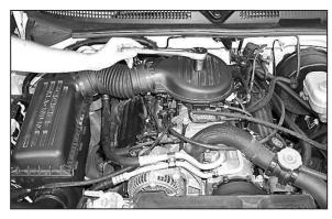
2. Loosen and remove the plenum retaining nut.
