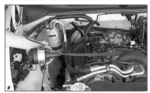
9. Remove the complete cruise control assembly.
