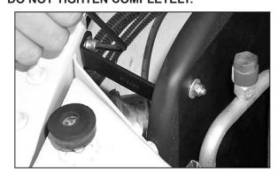
24. Attach the "C" bracket to the inner fender flange with the hardware provided as shown. **DO NOT TIGHTEN COMPLETELY.**
