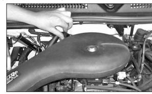
38. Reconnect the crankcase vent line to the K&N® intake tube as shown.
