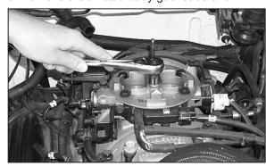
11. Loosen and remove the bolt that secures the stud/bracket assembly as shown.
