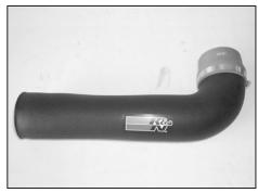
21. Install the silicone hose onto the  $K\&N^{\ensuremath{\$}}$  intake tube as shown
