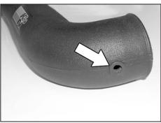
21b. Install the provided grommet into the intake tube as shown
