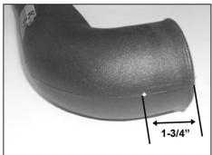
21a. On models that come equipped with an external temperature sensor, mark the intake tube 1-3/4" from the end of the tube, then drill a 3/4" hole into the intake tube.
