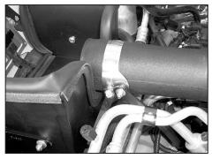
24. Secure the saddle bracket onto the K&N<sup>®</sup> intake tube with the provided hose clamp as shown.
