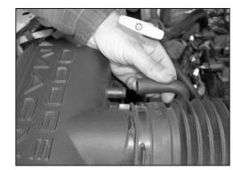
5. Remove the vent hose from the air box as shown.
