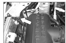
2. Loosen the hose clamp at the throttle body and air intake tube as shown.
