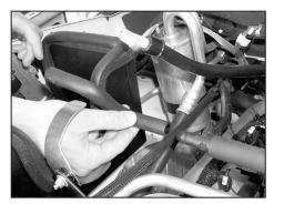
23. Remove the vent hose from the vehicle as shown.
