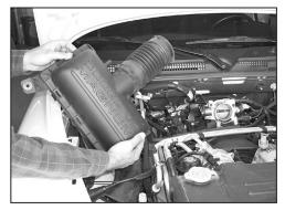
7. Pull firmly upwards on the stock air box to remove from the vehicle as shown. NOTE: K&N Engineering, Inc., recommends that customers do not discard factory <u>air intake</u>.
