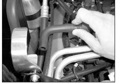
26. Re-install the vent hose onto the vent line as shown.
