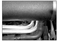
27. Connect the vent hose onto the  $K\&N^{\ensuremath{\circledast}}$  intake tube as shown.
