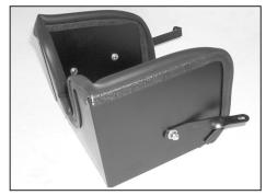
12. Install the provided twist bracket onto the heat shield as shown. Do not tighten completely.
