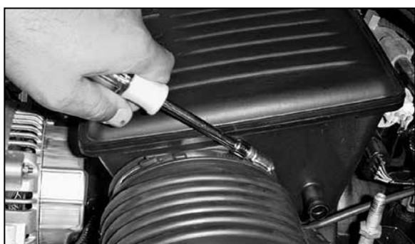
3. Loosen the hose clamp on the intake hose at the intake tube.
