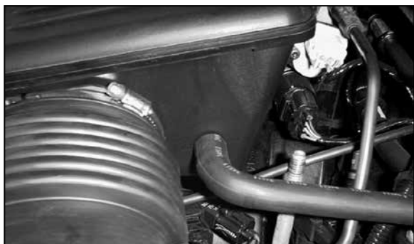
2. Detach the crankcase vent hose from the stock intake tube.
