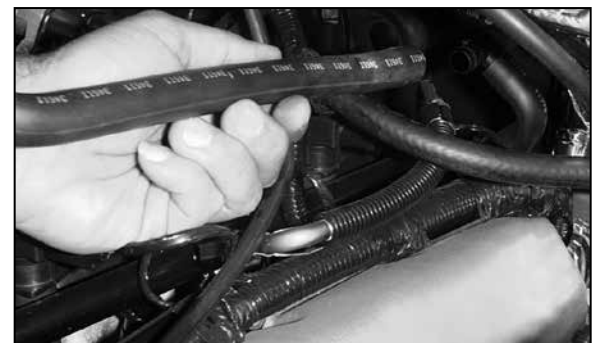
9. Detach the OE crankcase vent hose from the "T" fitting.
