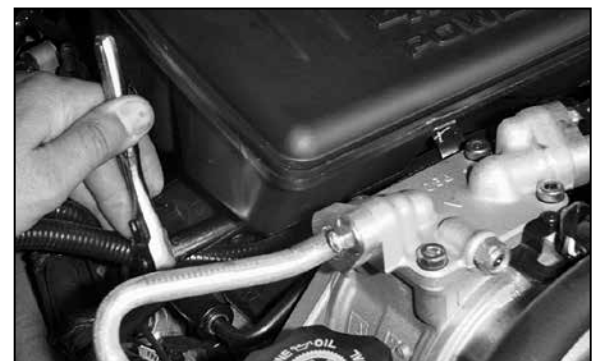
7. Loosen and remove the 2 bolts that retain the intake tube to the intake manifold.
