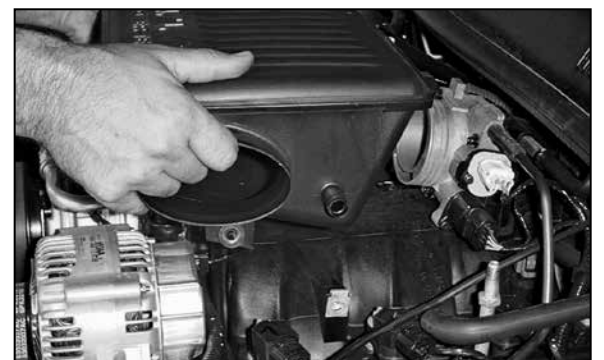
8. Pull firmly upward and remove the intake tube assembly.
