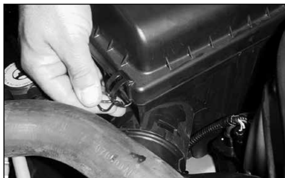
4. Release the 4 over center clips that retain the airbox top to airbox base.
