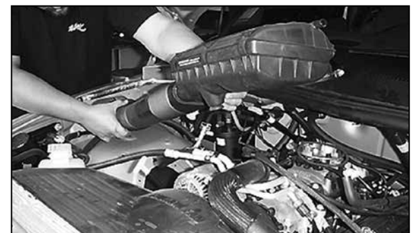
5. Detach the air inlet duct from the inner fender and remove the entire air cleaner assembly. NOTE: Remove the OE gasket as it will not be used.
