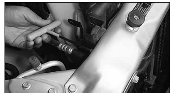
6. Mount the "Z" bracket to the existing hole in the radiator core support.
