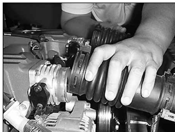
6. Disconnect the intake hoses from the throttle body.
