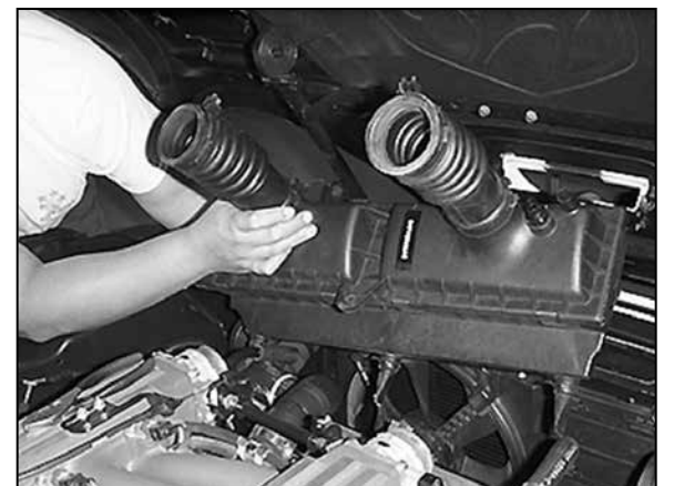
7. Remove the air box assembly. NOTE: K&N Engineering, Inc., recommends that customers do not discard factory air intake.
