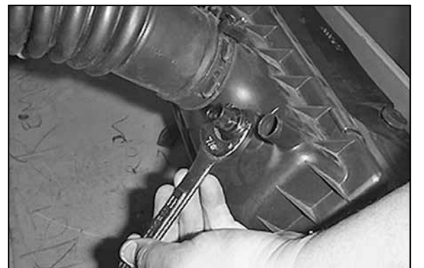
8. Loosen and remove the air temperature sensor from the air box.
