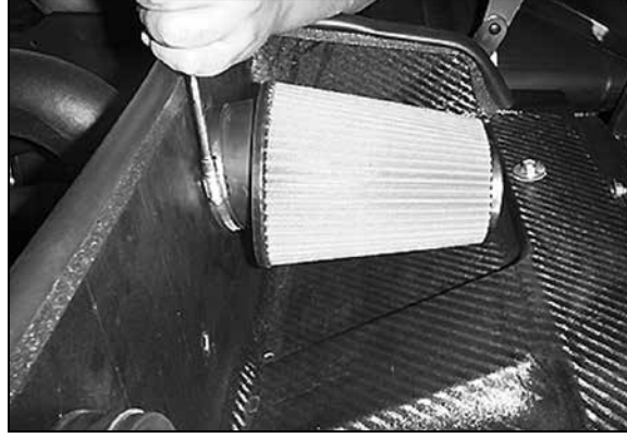
30. Install the K&N® air filter elements onto the intake tubes and secure with hose clamps.
