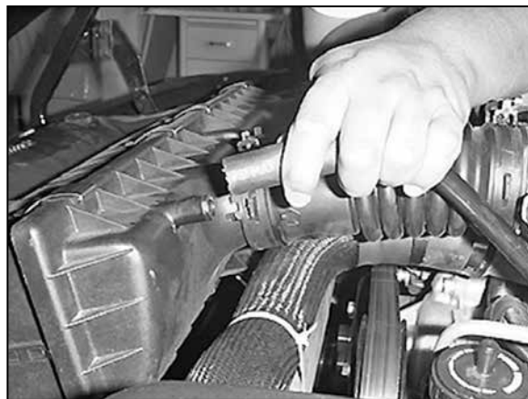
4. Detach the crankcase vent hose from the air box.
