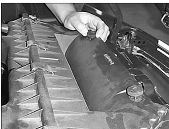
2. Loosen the three air box retaining screws, two in front and one in rear.
