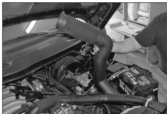
3. Unbolt the 10mm bolt at the bottom of fresh air intake tube then remove complete intake tube from vehicle.
