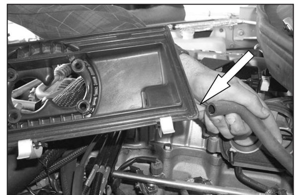
6. Disconnect crank case vent from air box base as shown. Then remove air box from vehicle. NOTE: K&N Engineering, Inc., recommends that customers do not discard factory air intake .
