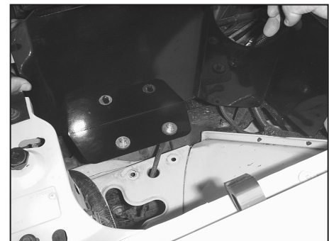
10. Install the heat shield with the provided hardware.
