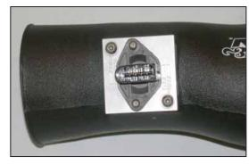
20. Secure the mass air sensor assembly into the K&N® intake tube with the provided hardware as shown.
