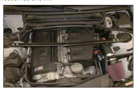
26. Re-install the strut tower brace that was removed in step 2.
