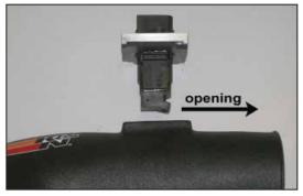
19. Install the mass air sensor assembly into the  $K\&N^{@}$  intake tube.
