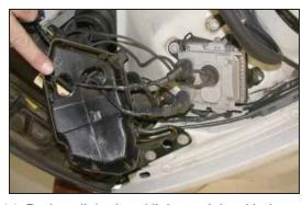
14. Re-install the head light module with the original hardware that was removed in step 5.NOTE: Install provided spacer under front mount as shown, then re-install module cover.
