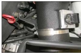
23. Attach the saddle bracket assembly to the intake plenum with the nut removed in step 9, then attach the saddle bracket to the intake tube with the provided hose clamp.
