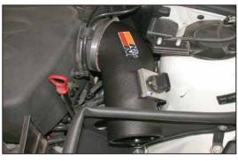
21. Attach the K&N® intake tube to the plenum with the provided hose clamp.
