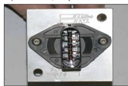
18. Install the mass air sensor into the mass air adapter as shown, secure with the provided hardware.
