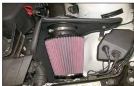
24. Install the K&N® air filter onto the K&N® intake tube and secure with the provided hose clamp.
