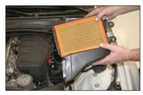
7. Remove the lower air box assembly as shown. NOTE: K&N Engineering, Inc., recommends that customers do not discard factory air intake.
