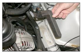
10. Pull up the lower air box locator to remove it from the mounting studs and then from the vehicle.
