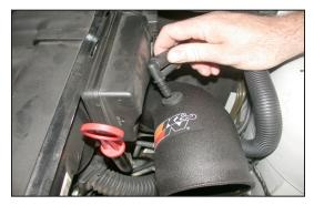
13. Insert the factory vent tube into the grommet in the intake tube as shown.
