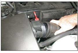
4. Loosen then hose clamp which secures the factory intake tube to the mass air sensor, then disconnect the intake hose from the mass air sensor as shown.
