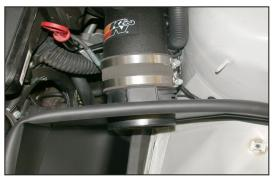
21. Install the mass air sensor assembly into the heat shield and onto the K&N® intake tube, secure with the provided hose clamp.
