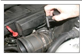
7. Pull up on the vent tube to dislodge it from the intake tube as shown.
