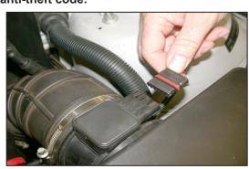
2. Release the locking tab and disconnect the mass air sensor electrical connection.
