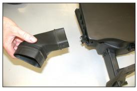
15. Remove the fresh air duct from the air box as shown.
