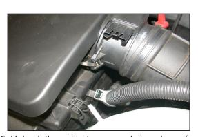
5. Unhook the wiring harness retainer shown from the rear of the box.
