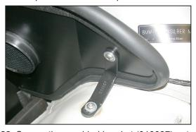
22. Secure the provided bracket (010087) onto the heat shield and inner fender with the provided hardware as shown.
