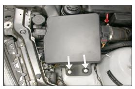
3. Remove the two factory air box mounting bolts shown.
