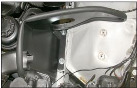
17. Install the heat shield assembly into the vehicle and secure with the provided fender washers and 6mm nuts onto the lower air box mount studs. Reinstall the fresh air hose into the fresh air duct.
