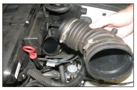
8. Loosen the lower hose clamp, which secures the upper intake tube to the lower intake tube, and then remove the upper intake tube from the vehicle.
