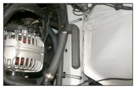
9. Unclip the rubber strap, which secures the heater hose to the lower air box locator.
