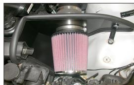
23. Install the air filter onto the mass air sensor and secure with the provided hose clamp.
