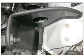
18. Reinstall the lower air box locator removed in step #10 and resecure the heater hose.
