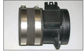
20. Install the silicone hose (08630) onto the mass air sensor and secure with the provided hose clamp.
