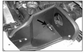
16. Install the heat shield assembly onto the vehicle.
