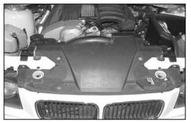
23. Re-install the radiator cover removed in step #9 and secure with the existing hardware.
