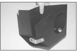
14. Install bracket (070015) onto the heat shield with the provided hardware as shown. **NOTE: Do not tighten at this time.**
