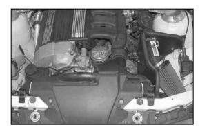
24. Reconnect the vehicle's negative battery cable. Double check to make sure everything is tight and properly positioned before starting the vehicle. 25. It will be necessary for all K&N<sup>®</sup> high flow intake systems to be checked periodically for realignment, clearance and tightening of all connections. Failure to follow the above instructions or proper maintenance may void warranty.
