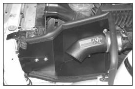
19. Install the intake onto the mass air sensor, then secure with the provided hose clamp and secure the tube mounting bracket to the heat shield with the provided hardware.
