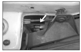
10. Using a flat blade screwdriver, unhook the fresh air duct behind the head light.
