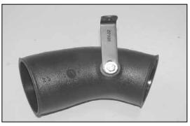
18. Install the tube mounting bracket (07195) onto the intake tube with the provided hardware.
