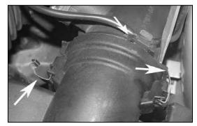
4. Using a flat blade screwdriver, unlock the mass air sensor retaining clips as shown.
