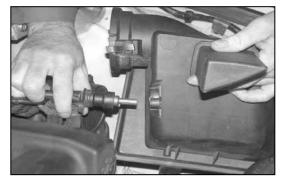
6. On vehicles equipped with a throttle body heater, lift the air box partially out to access throttle body heater thermostat. Remove the retaining bolt, then remove the thermostat from the air box as shown.
