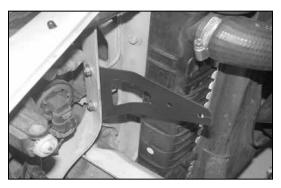
13. Install the heat shield mounting bracket onto the existing holes of the radiator core support with the hardware provided as shown.
