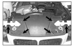
8. Remove the four screws shown that secure the radiator cover in place, remove the two plastic retainer clips by pulling up on the center pin.
