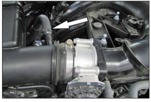
3. Release the spring clamp and disconnect the crank case vent hose from the factory intake tube.
