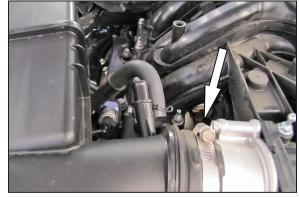
4. Loosen the hose clamp securing the factory intake tube to the throttle body.
