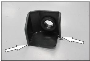
11. Install the provided edge trim onto the  $K\&N^{\otimes}$  heat shield as shown.
