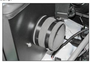
14. Install the provided step coupler (08496) onto the filter adapter and secure with the provided hose clamp.
