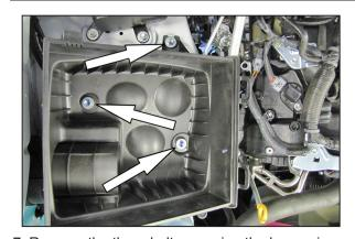
7. Remove the three bolts securing the lower air filter housing to the inner fender and then remove the lower air filter housing from the vehicle.
