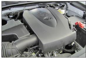
2. Lift up the engine cover to dislodge it from the mounting studs and then remove it from the vehicle.
