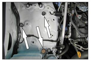
8. Install the three provided rubber mounted studs onto the inner fender in the positions shown.
