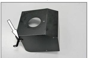
9. Install the provided heat shield bracket (07958) onto the  $K\&N^{\otimes}$  heat shield as shown.
