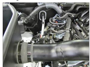
20. Reconnect the mass air sensor electrical connection.
