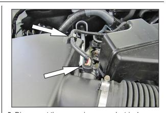
5. Disconnect the mass air sensor electrical connection and unhook the harness from the air filter housing.
