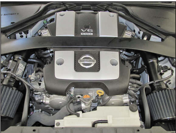
41. Adjust the intake tubes for uniform fit and then reinstall the engine cover and secure with the factory bolts.
