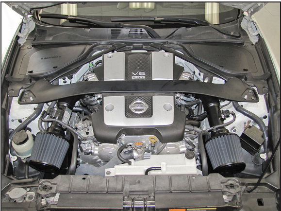
42. Reconnect the vehicle's negative battery cable. Double check to make sure everything is tight and properly positioned before starting the vehicle.
