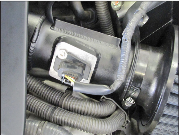
40. Reconnect the mass air sensor electrical connection.
