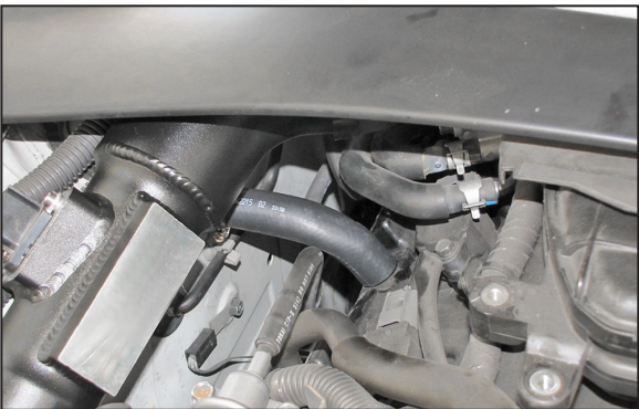
38. Install the 5" crank case vent hose onto the 90° fitting on the K&N® intake tube and then attach the open end to the vent port on the valve cover.
